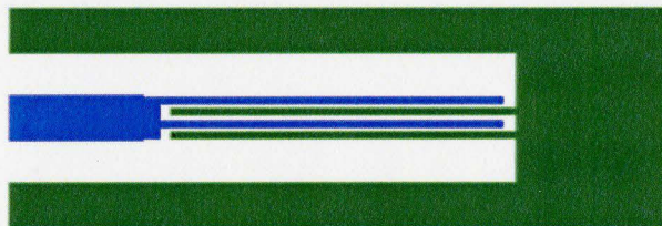
Figure 14: Top view of interdigital circuit design
