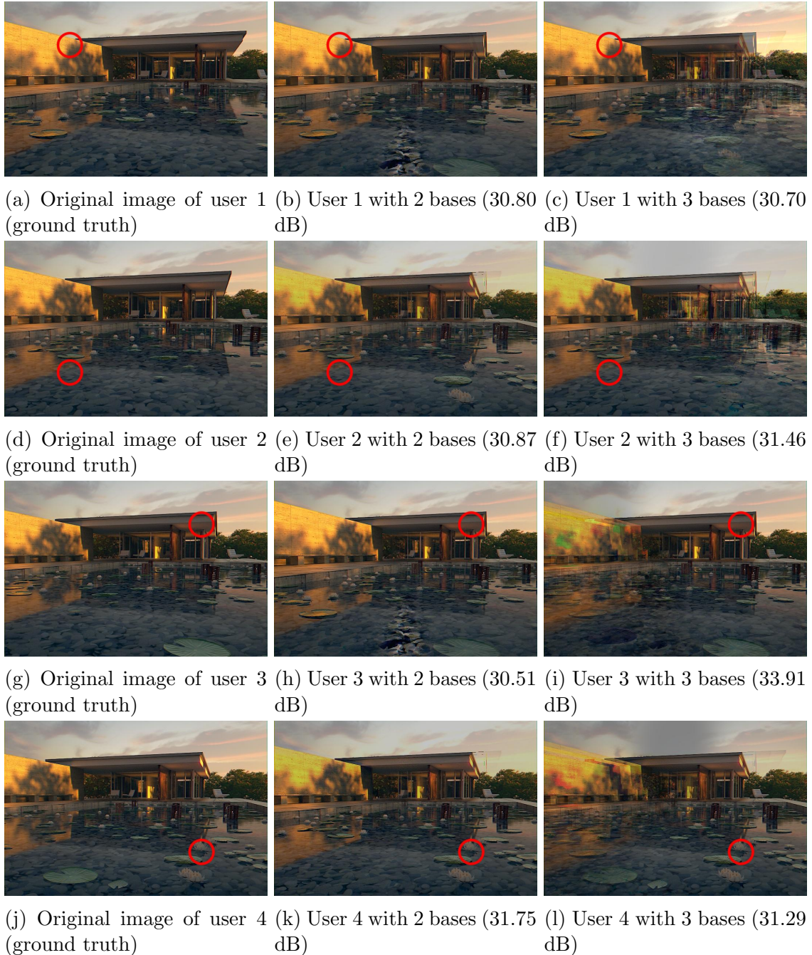
Figure 4.2: Results of fovea weighting of TPVM in the pavilion scene. The red circles indicate the centers of regions of interest of different users. The PSNRs reported are fovea weighted PSNR.
