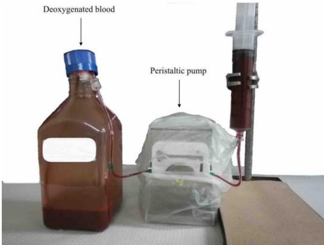
Figure 4.7 – Experimental setup to load the syringes with blood. Blood with low O 2 concentration was pumped into a 60 mL syringe at maximum speed.
