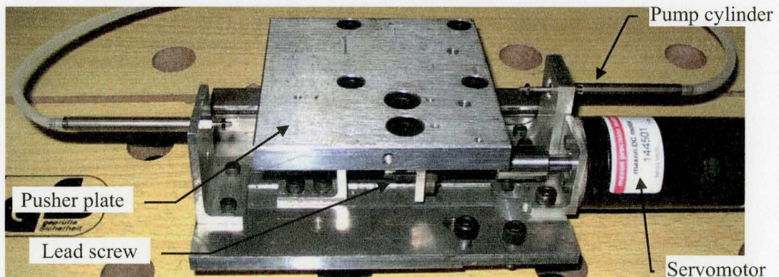
Figure 3.8.1: First prototype of motor-cylinder pump
