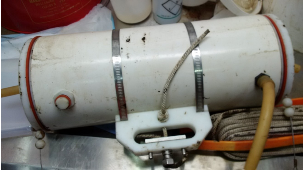
Figure 2-5: Van Dorn used to collect water for all geochemical sampling.
