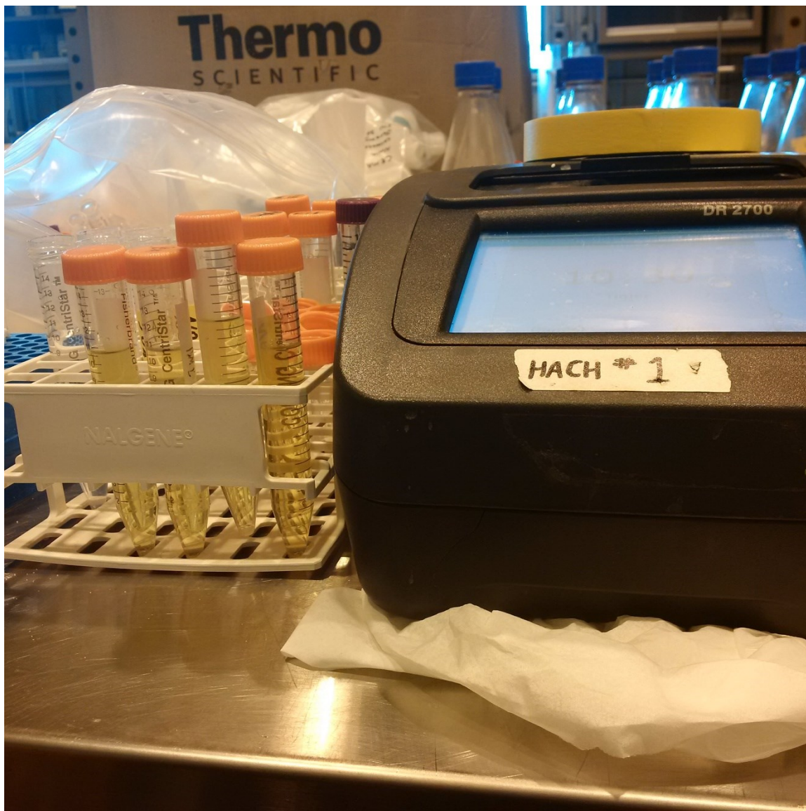
Figure 2-7: Ammonia analysis following the HACH method 8155.
