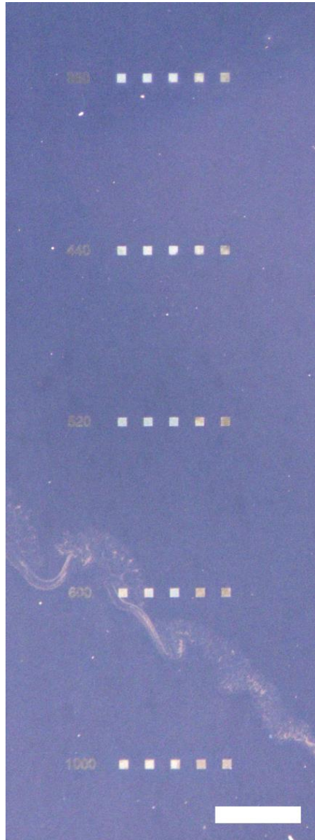
Figure 6-3: Light microscope image of sample #1849 after nw growth, showing a single column of the EBL pattern; this column is repeated three times per wafer to produce a total of 75 separate 100\ \mu\text{m} \times 100\ \mu\text{m} nw pads (white squares). Scale bar is 1 mm.
