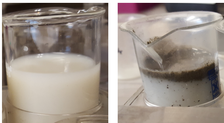
Figure 24: The picture on the left shows a “wastewater 1” sample after removing the insoluble oil layer from the top. This was done after letting the sample sit for 10 – 15 minutes for the oil to float to the top and be removed. The picture on the right shows “wastewater 1” as received from Aevitas before any treatment.
