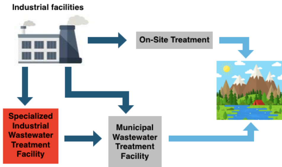
Figure 1: Schematic that illustrates the different routes that wastewater can go through from the generator to the environment
