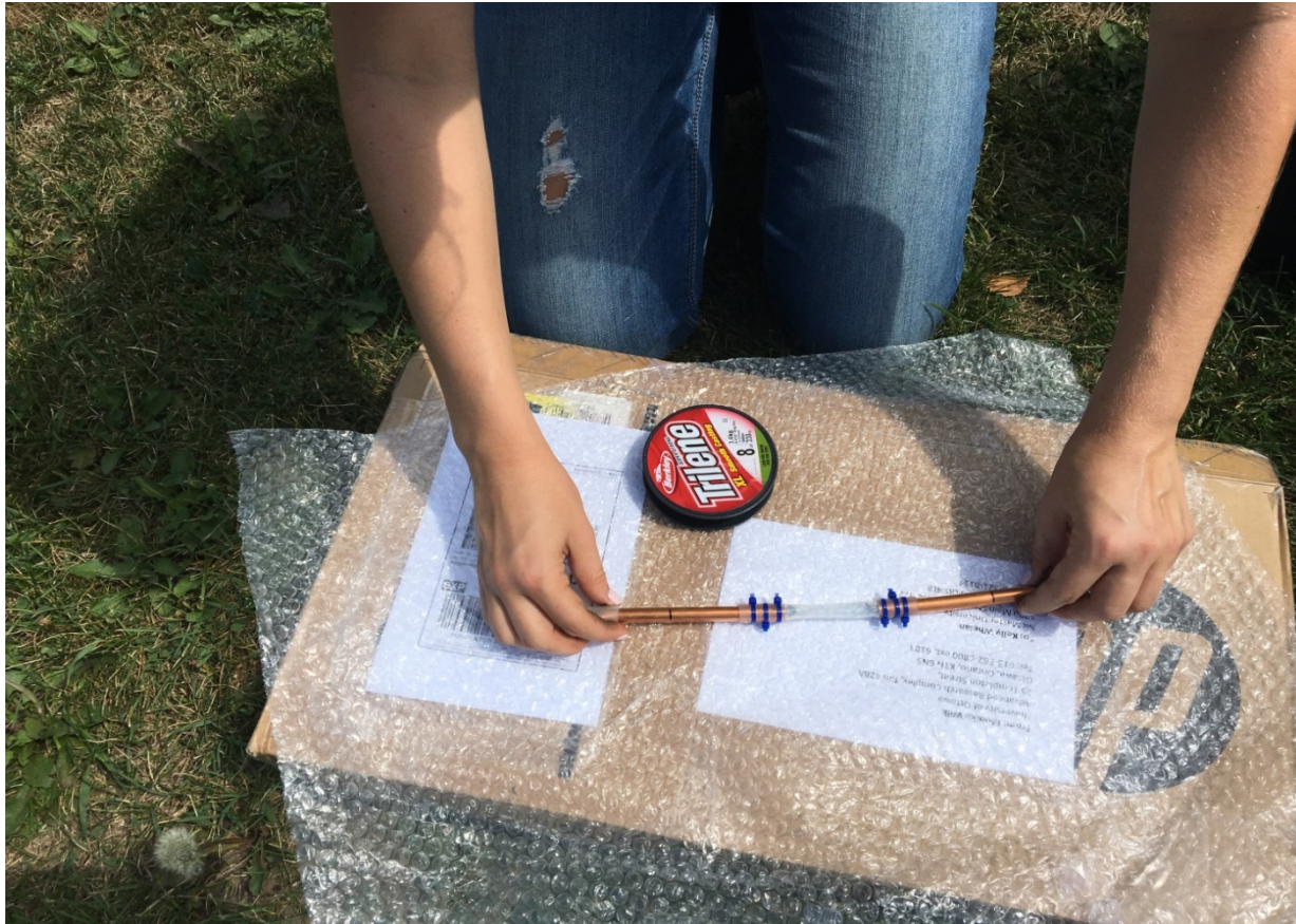
Fig. A6: Copper and Silicon tube diffusion samplers used from collecting helium concentration from groundwater.
