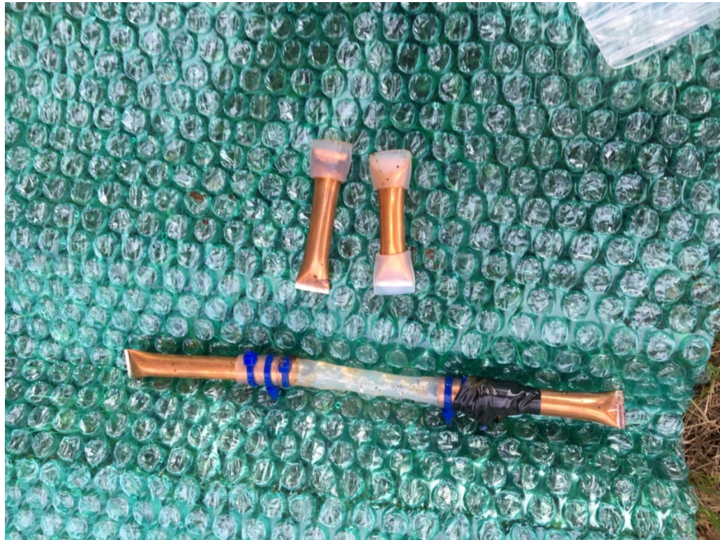
Fig. A9: Copper and Silicon tube diffusion samplers after crimping occurred. Plastic silicon ends were placed on crimped area to avoid damage or opening of sampler during shipping.
