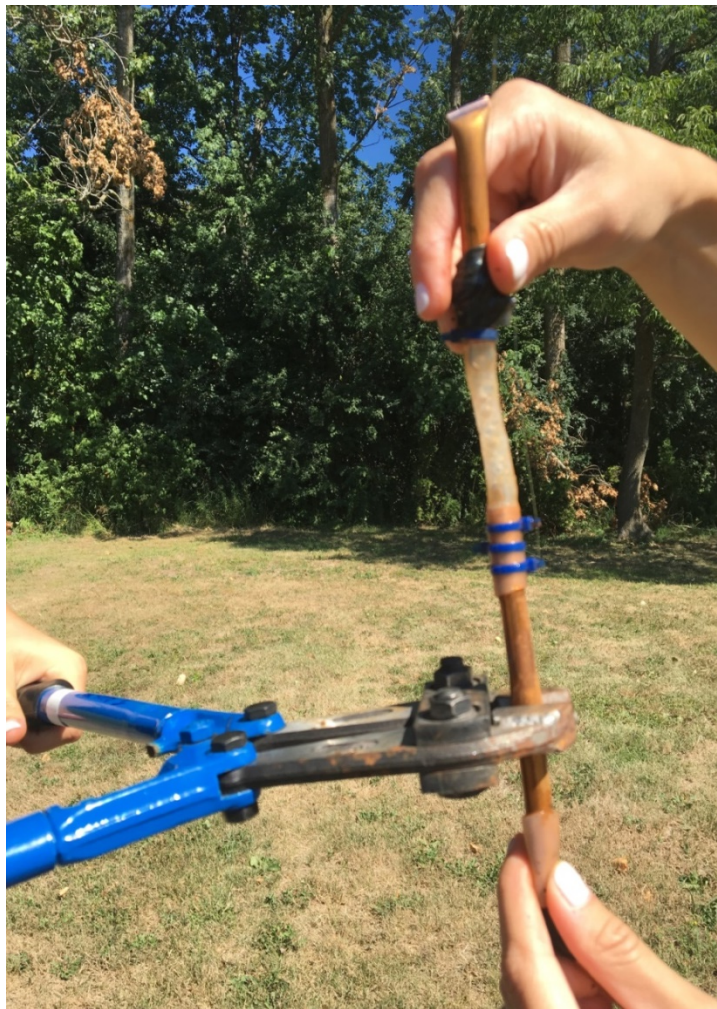
Fig. A8: Crimping of copper tube diffusion samplers used for collected helium concentration in groundwater
