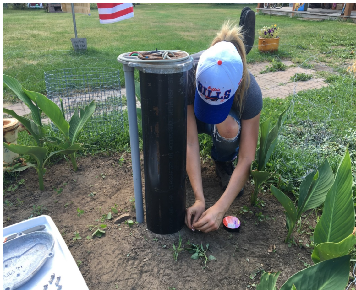
Fig. A7: Diffusion samplers anchored outside of the well and suspended from fishing line.
