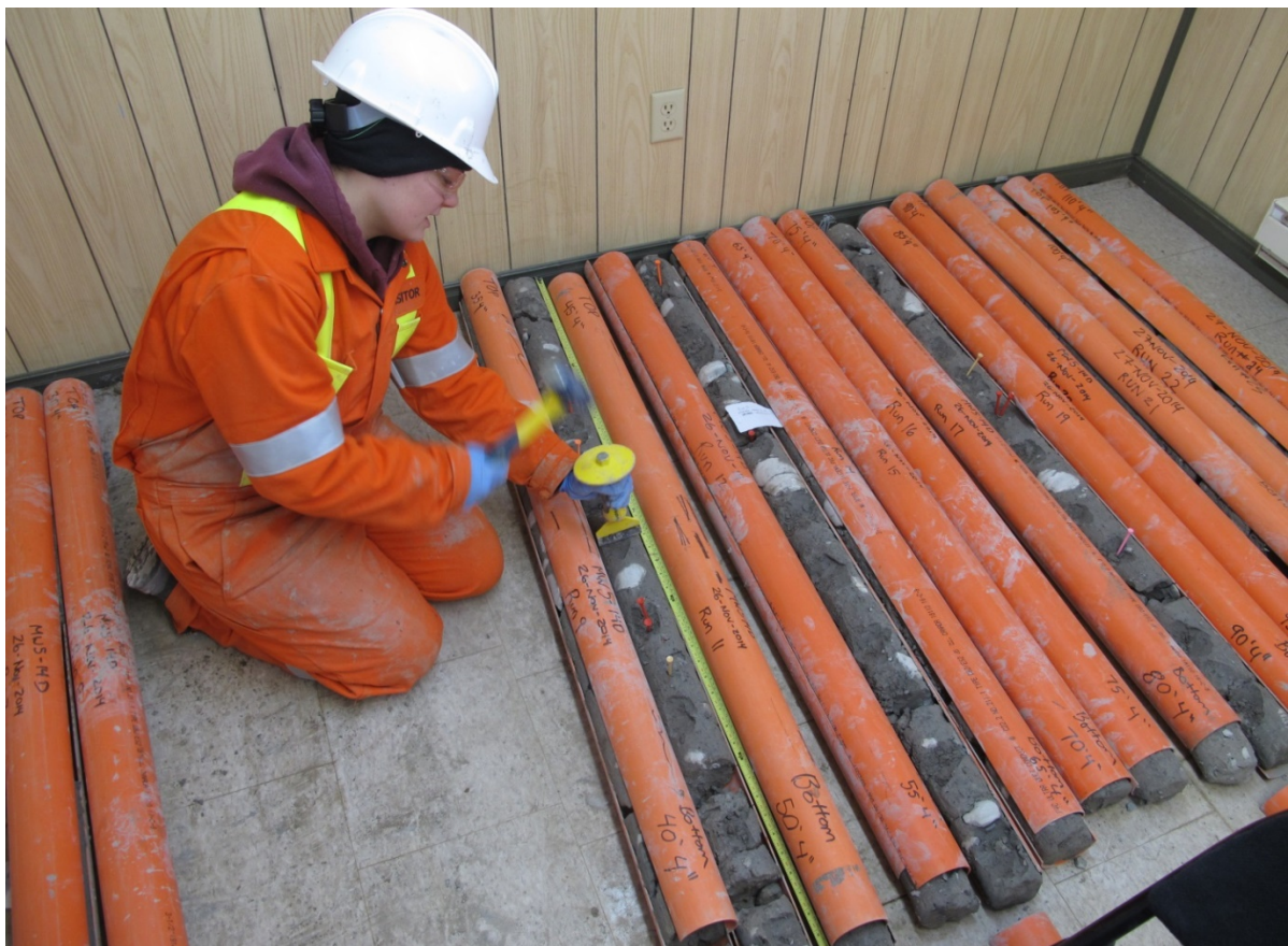
Fig. A4: MW5-14D grain size sampling with hammer and chisel where Newmarket Till became very dense. Grain size samples were collected in approximately six (6) inch cores.
