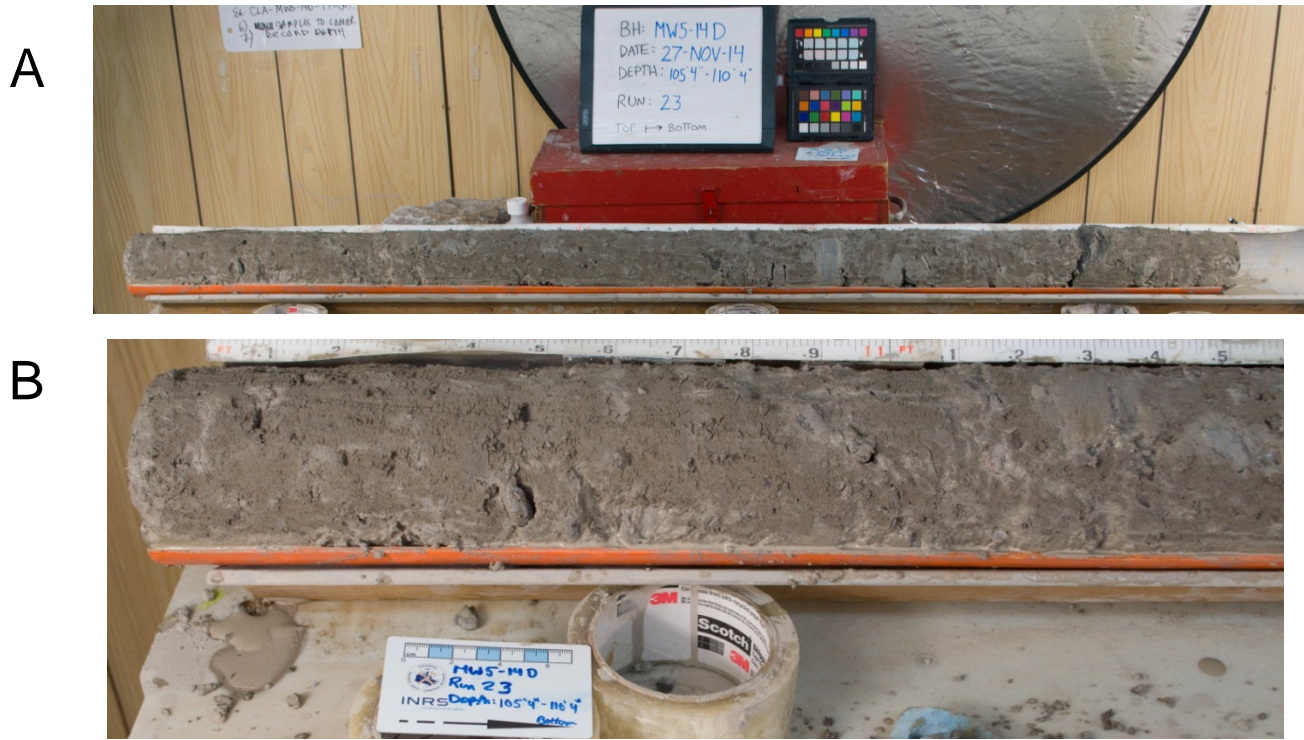
Fig. A1: (A) MW5-14D 5 foot run section of diamict, with reference color card (passport colorchecker) located to the right of the marker board. (B) MW5-14D 1 foot detailed section of diamict.
