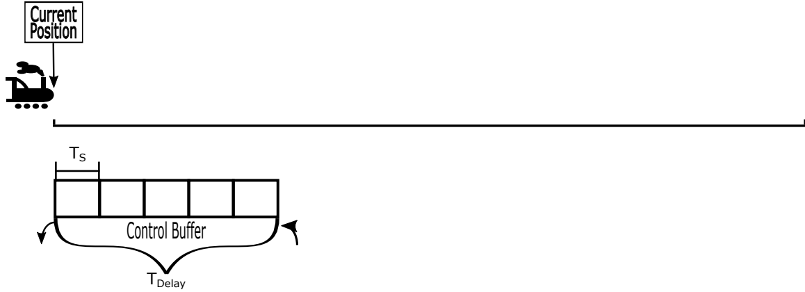
Figure 5.1: Control buffer. The arrow pointing into the control buffer shows where the control commands enter the buffer, and the arrow pointing out of the control buffer shows where the control commands exit the buffer.
