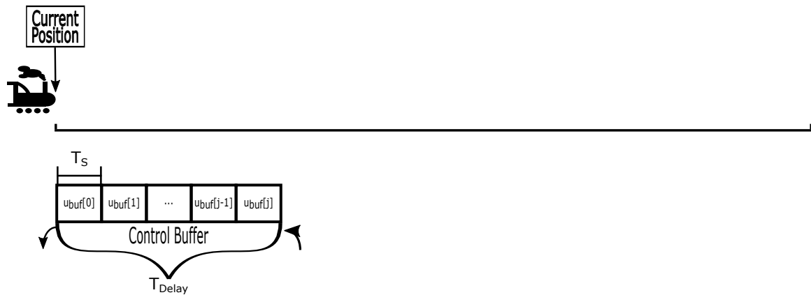
Figure 5.4: Control buffer filled.
