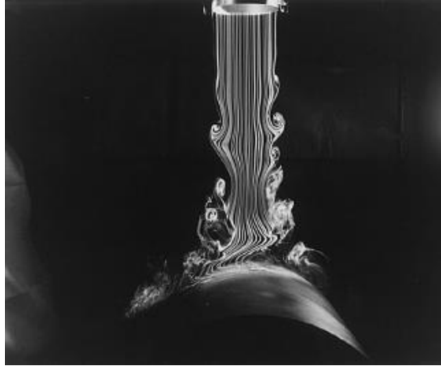
Figure 1.5: Impingement on a convex surface ( Re = 6000 , H/d = 4 ) (Cornaro, Fleischer, & Goldstein, 1999)
