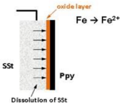
Fig 2-14 The formation of iron oxalate layer [66]
