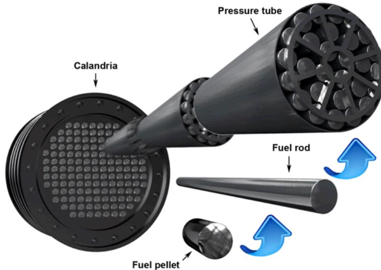
Figure 1: Displays CANDU reactor calandria and other components from [1]
