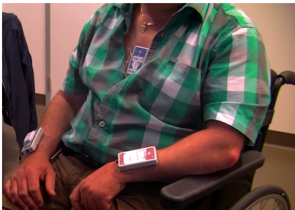
Figure 3. Positioning of the Activ8 and VitaMove AMs on wheelchair users.
