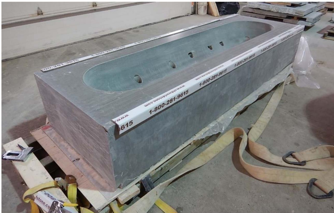
Figure 1.4: Shaping trial of a full-sized HCB clay buffer block (Crowe, 2016).
