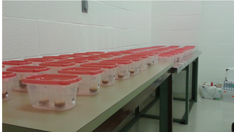
FIGURE A1.2: The Snaptite chambers in the controlled room with little disturbances, with controlled light, air, temperature and humidity
