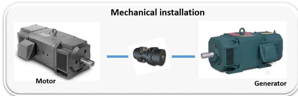
Figure A.1: Motor lab mechanical installation
