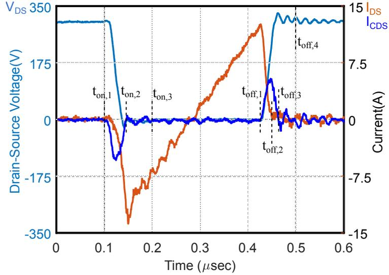
Figure 4.4: Waveforms for the turn-on and turn-off of  $M_2$  with use of additional 330pF capacitor with the MOSFETs.
