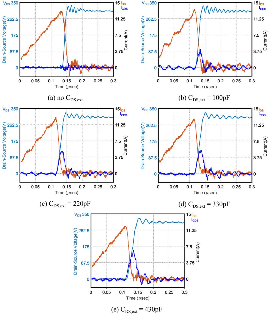
Figure 4.6: Waveforms for the turn-off of  $M_2$  with use of additional capacitors across the MOSFETs' drain-source terminals.
