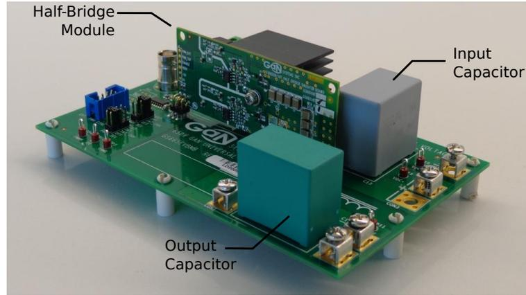
Figure 4.7: Buck converter experimental hardware.
