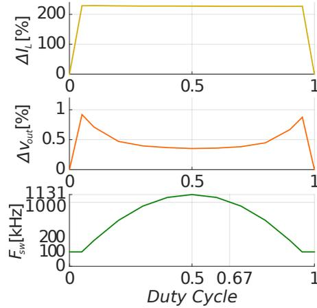
Figure 4.3: Variation in inductor current ripple, output voltage ripple and switching frequency with change in duty cycle in a buck converter using linear SSW.
