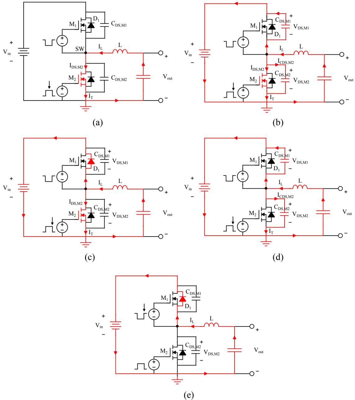
(a) Current conduction when  $M_2$  is ON (b) when  $I_{DS,M2}$  is reducing and additional capacitors are charging during  $t_{off,1}-t_{off,2}$  (c) when  $V_{DS,M2}$  reaches  $V_{in}$  before  $I_{DS,M2}$  reduces to zero (d)  $I_{DS,M2}$  reaches zero while current flows through the additional capacitors during  $t_{off,2}-t_{off,3}$  (e) completion of turn-off of  $M_2$  and reverse conduction through  $M_1$  during  $t_{off,3}-t_{off,4}$ .
