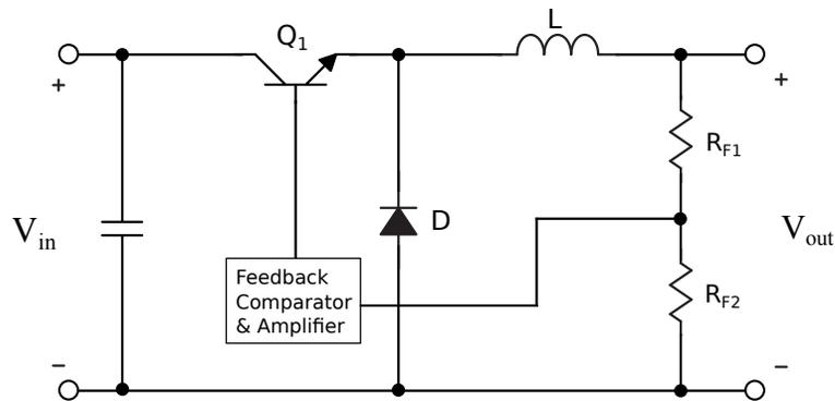
Figure 1.3: Buck Converter Topology
