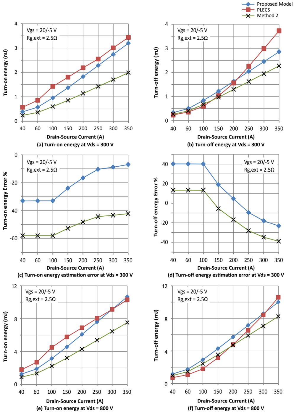
Figure 2.4: Comparison of switching energy values and errors from proposed model, *Method 2* and PLECS simulation
