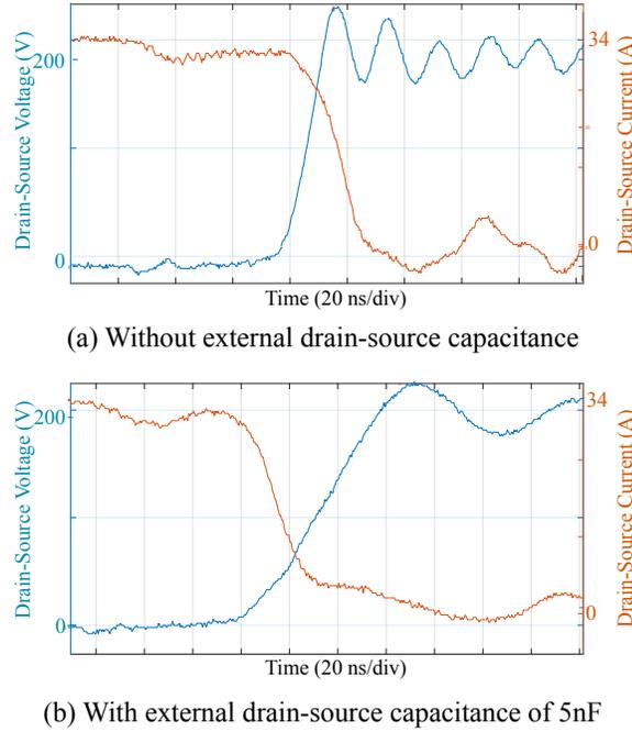
Figure 3.7: Switching waveforms for turn-off of  $M_2$  for test conditions in Table 3.1.
