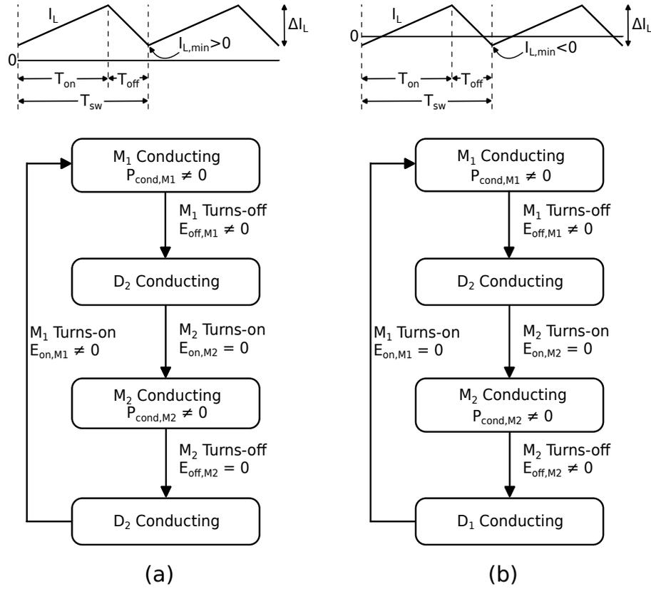
Figure 4.1: Switching events and the associated losses during a switching time period in a buck converter using GaN devices with (a)  $I_{L,min} > 0$  (b)  $I_{L,min} < 0$ .
