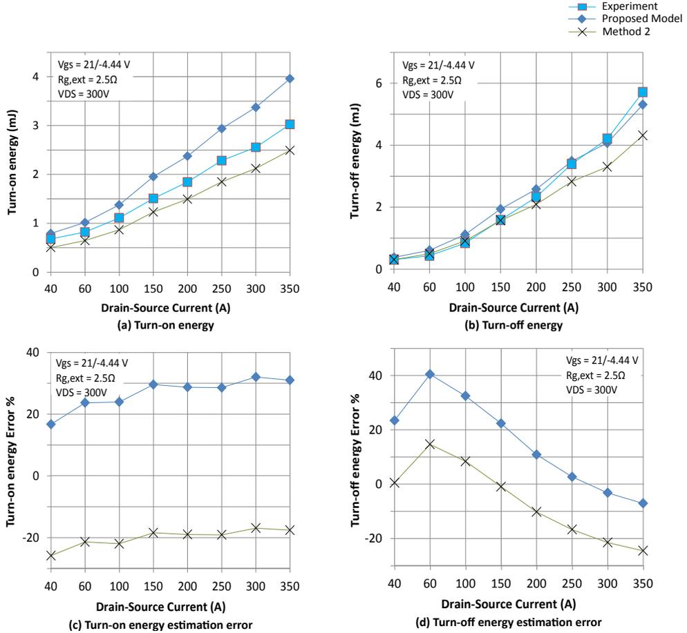
Figure 2.6: Comparison of switching energy values and errors from proposed model, *Method 2* and double pulse test experiment
