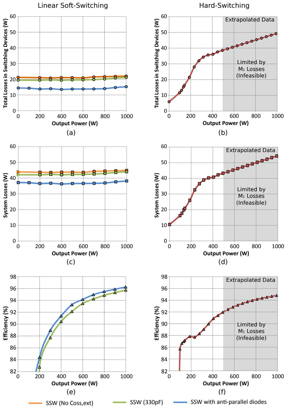
Figure 4.10: Losses and efficiency in a buck converter at 1MHz switching frequency with linear soft-switching and hard-switching.
