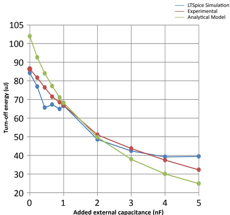
Figure 3.6: Reduction in turn-off losses
