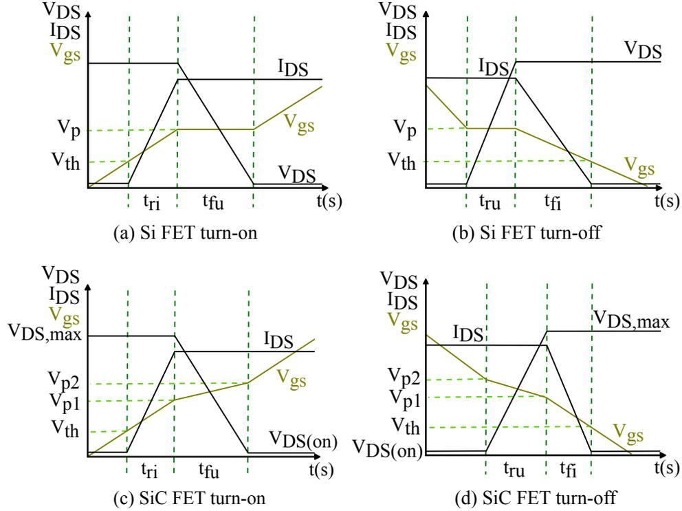
Figure 2.1: MOSFET Switching characteristics
