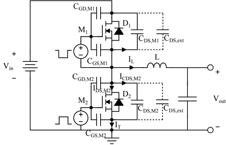
Figure 3.1: Buck Converter Topology
