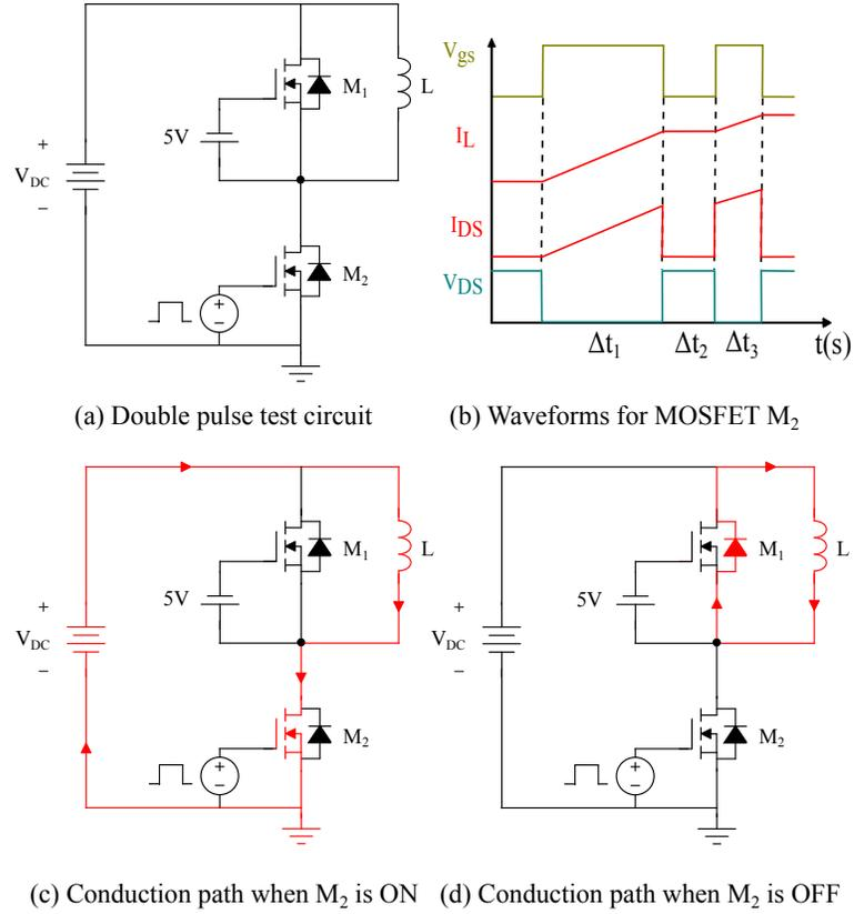
Figure 2.5: Double pulse test circuit and waveforms.
