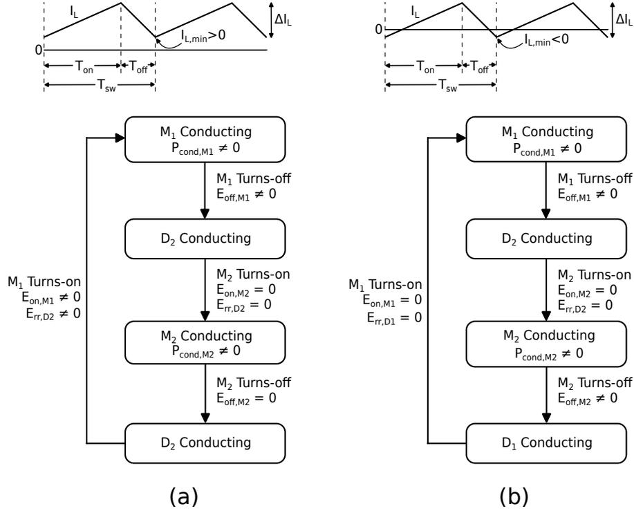
Figure 3.2: Sources of power loss during a switching cycle for a buck converter with (a)  $I_{L,min} > 0$  (b)  $I_{L,min} < 0$ .
