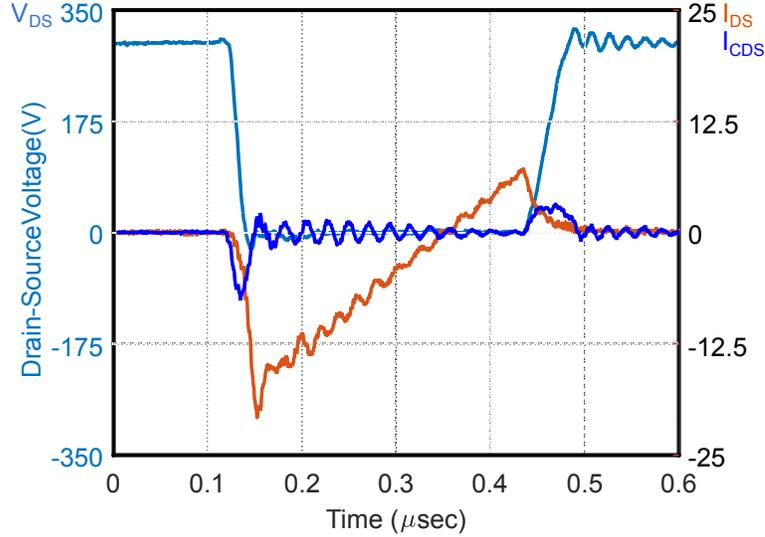
Figure 4.9: Waveforms for the turn-on and turn-off of  $M_2$  with use of additional 330pF capacitor with the MOSFETs in the buck converter at 1kW output power.
