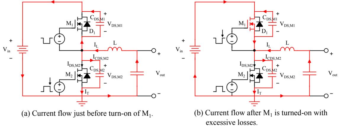
Figure 4.2: Buck converter using large additional capacitors with MOSFETs and small dead-time
