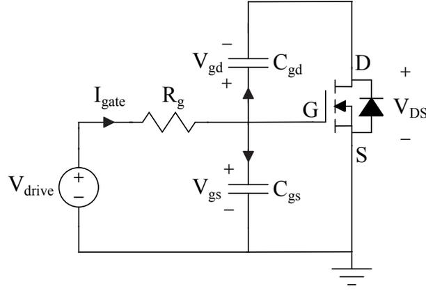
Figure 2.2: MOSFET gate charging and discharging equivalent circuit
