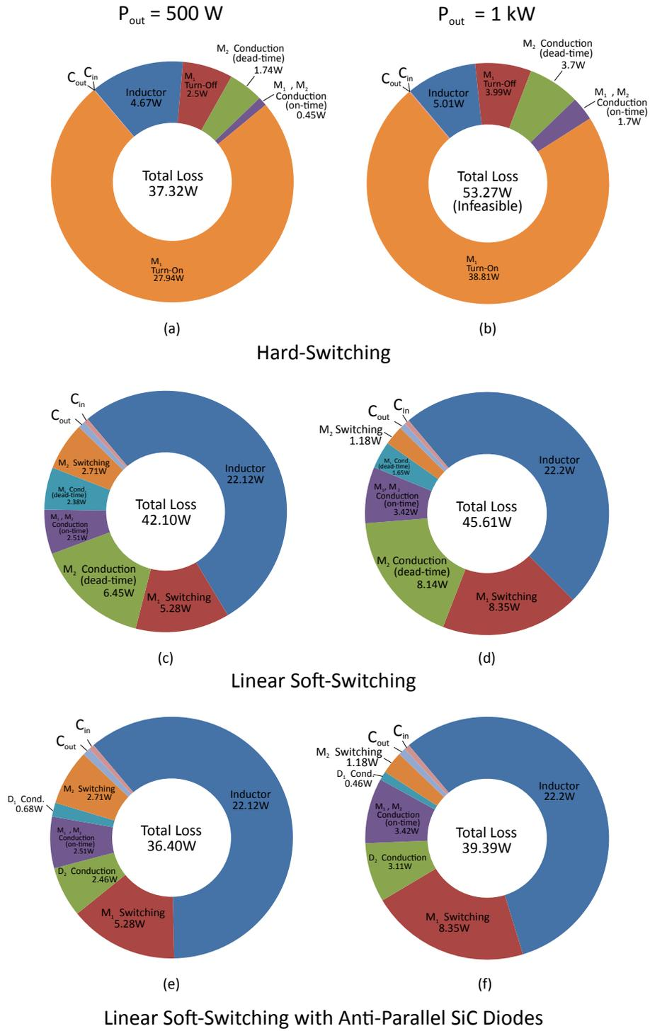
Figure 4.11: Power loss estimation using analytical calculations and models at 1MHz for different  $P_{out}$ .
