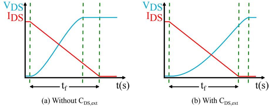
Figure 3.3: Representative waveforms for voltage across and current through  $M_2$  at turn-off.
