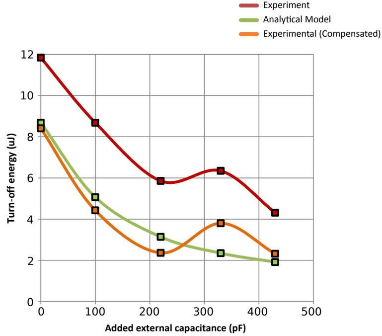
Figure 4.8: Reduction in the turn-off losses using the analytical model and in experiment (with and without effect of current in the FET inherent parasitic capacitance)
