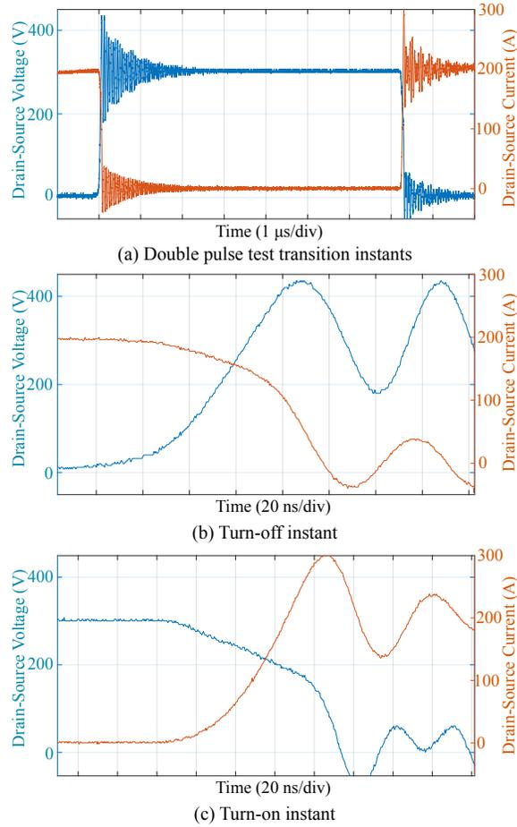
Figure 2.7: Switching waveforms for  $V_{DS}=300\text{V}$ ,  $I_{DS}=200\text{A}$
