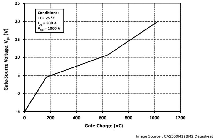
Figure 1.5: Varying Miller Plateau Voltage
