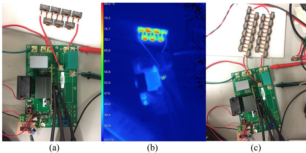
(a) Top-view of the buck converter board using 2.1  $\mu\text{H}$  inductor and the linear SSW method (b) Thermal image for operation of the top system at 1 kW with forced air cooling at 27°C (c) Top-view of buck converter using 20.7  $\mu\text{H}$  inductor and hard switching. Its steady-state thermal image is not captured to avoid system failure due to large switch losses and the resultant heating.
