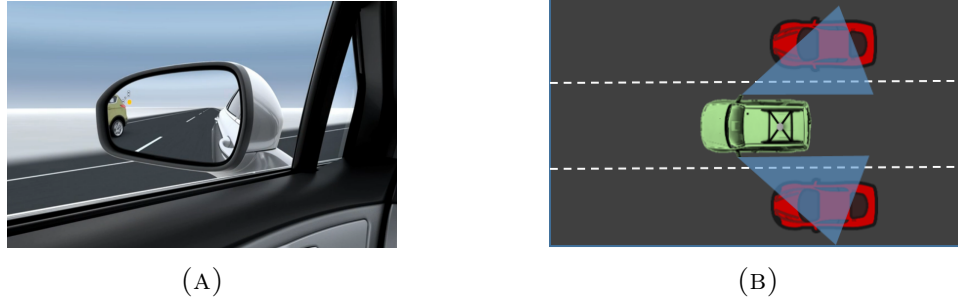
FIGURE 1.3: Ford's blind spot information system
