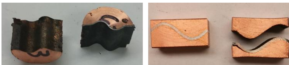
Figure 5-62: Photographs of samples that failed at the interface prior to successful testing. (Left) Picture of copper-IF steel sample that broke apart at the interface during machining. (Right) Picture of copper-GP1 steel sample, with a before and after shot of samples, that broke apart at the interface during rolling.
