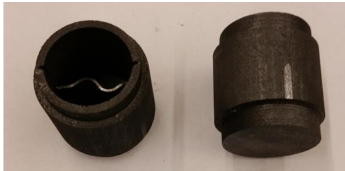
Figure 5-61: Photograph of graphite casting crucibles used to cast copper matrix composites. (Left) A crucible loaded with a corrugated strip and (right) a crucible on its side showing the indents used for balancing the quartz tubes.
