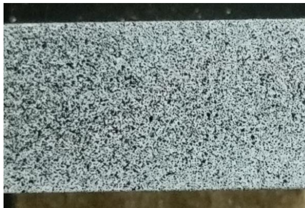
Figure 5-27: Spray paint generated, random pattern used for Digital Image Correlation.
