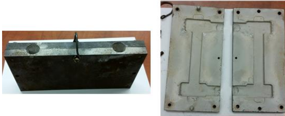
Figure 5-21: Die used for casting dog-bone composite samples in assembled (left) and open (right) configurations.
