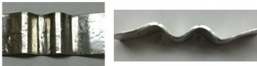
Figure 5-20: Copper strip after pre-coating of solder has been applied.
