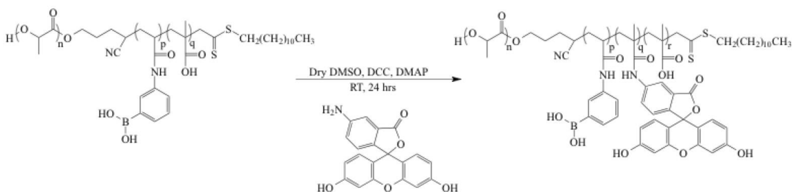
Figure 11 - Carbodiimide-mediated coupling of 5-fluoresceinamine to micelle copolymer
