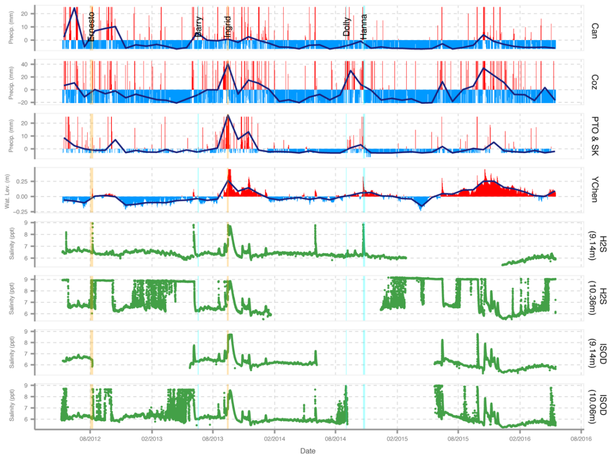
Fig. 3 – Time series plots from May 2012 to 2016 (GMT) for: 1) precipitation (mm) from Cancun, Cozumel and Sian Ka’an and Puerto Aventuras weather stations; 2) Yax Chen groundwater level (m) and salinity (ppt) from the two monitoring sites (H2S, -9.14 and -10.36 m depth; ISOD 2, -9.14 and -10.06 m depth). Precipitation and water level are plotted as departure from the mean over the analysis period while salinity (ppt) is plotted as 30-min time intervals. Monthly trends are also plotted which are monthly mean departure values. Gaps in the records are due to sensor malfunction and battery depletion, and flat-lined data (salinity) is due the sensor going out of range (>9 ppt). Hurricanes (orange) and tropical storms (blue) are highlighted over the analysis period.
