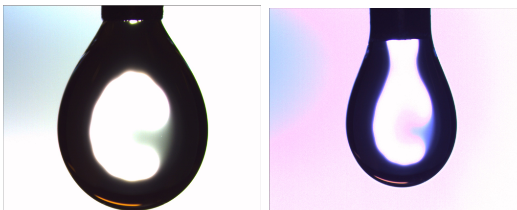
Figure 4-11. Pendant drop images obtained during CMC measurements for water (left) and compound 2 (allyl-PEG-TES) at a concentration of 0.1 w/v % in distilled water (right). Note these pictures are not to scale, however, the difference in droplet curvature resulting from the differences in surface tension of the liquid is apparent.
