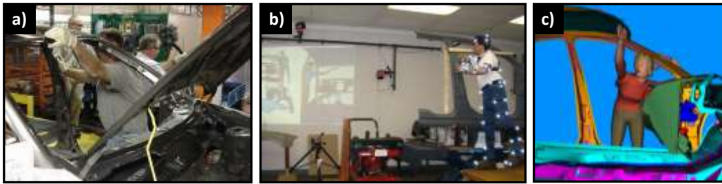
Figure 3: Sample of the process by which an assembly-line task (a), was simulated in a laboratory setting (b). A subject was equipped with a motion tracking suit (i.e. reflective markers) and performed the task as if they were on the assembly-line, with physical props and virtual feedback. The motion data were then streamed into the Jack software (c) where the motion data drive the manikin’s movement. The postural data from the manikin are used to assess joint injury risks using ergonomic tools.
