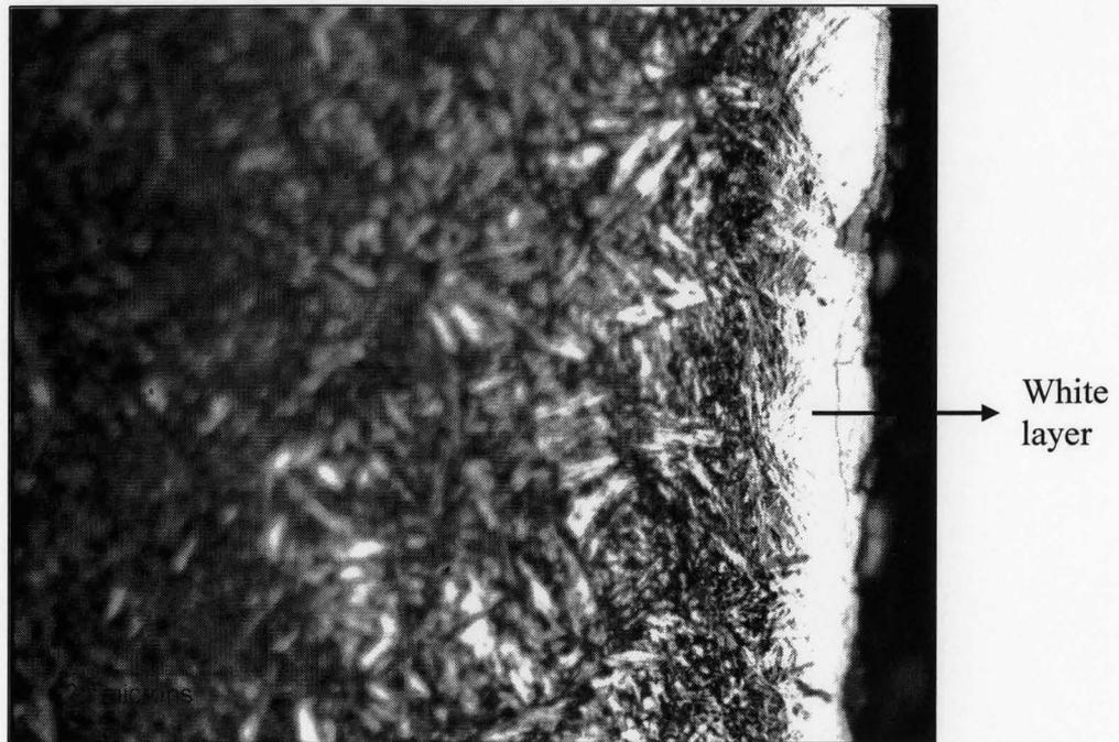
**Figure 4.2.** A photomicrograph of white layer of thickness  $16.38\mu\text{m}$  from sample NN29S92 (x1000).
