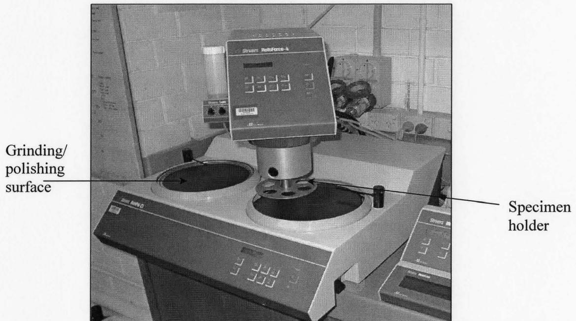
**Figure 3.11** STRUERS ROTOPOL-2 grinding /polishing machine
