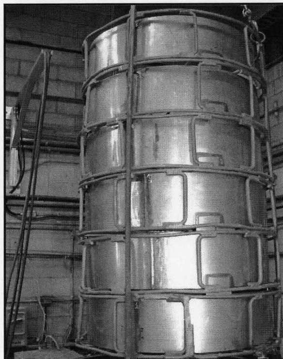
**Figure 2.8:** A general view of load basket with liner
