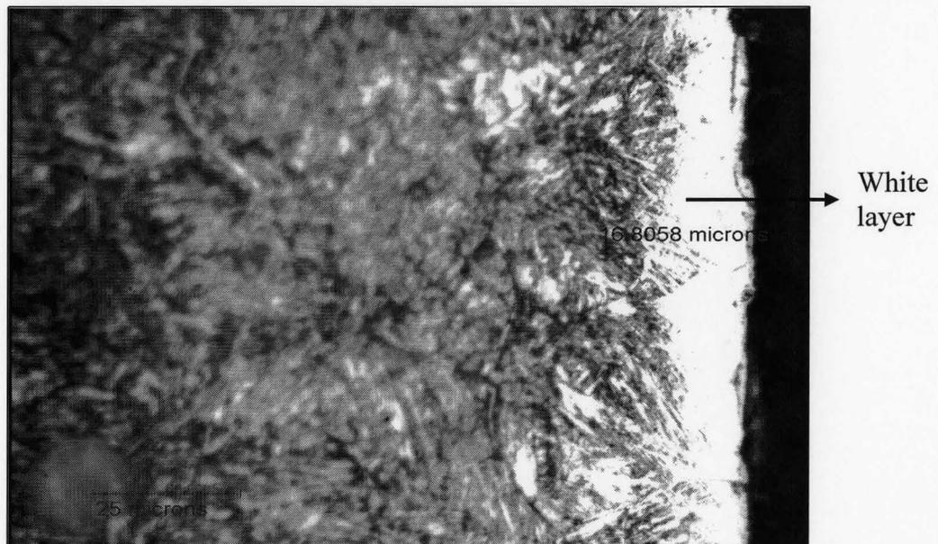
**Figure 4.3:** A photomicrograph of white layer of thickness  $16.06\mu\text{m}$  from sample NN39S122 (x1000).
