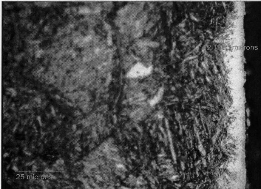
**Figure 3.17.** A photomicrograph of sample “NN32S013” nitrided for 20 hrs at a  $K_N$  thickness of 0.45 and 1050 °F. White layer thickness is about 12.11  $\mu\text{m}$  (x1000).
