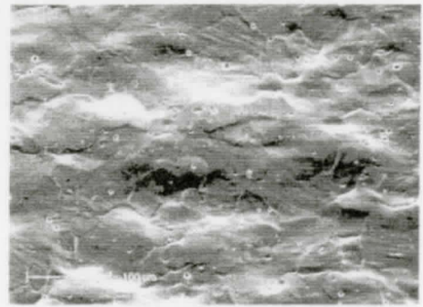
(b) Tested Perpendicular to Rolling Direction to 24% strain
