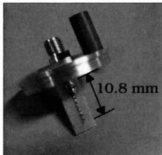
Figure 2.12, Photograph of Wu-King monopole antenna [19].
