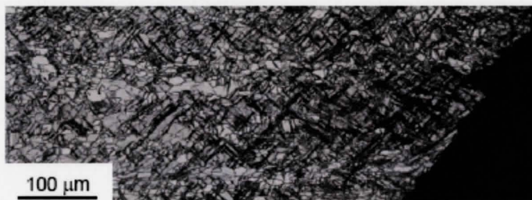
Figure 2.17 Twinning and shear bands in AZ31 at fracture (Barnett (2007)).
