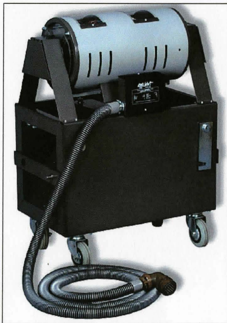
Figure 4.1: Four-pole squirrel-cage induction machine – Model 8503
