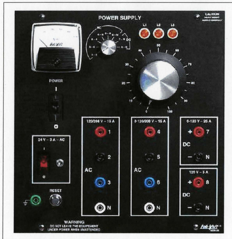
Figure 4.5: The power supply module - Model 8525
