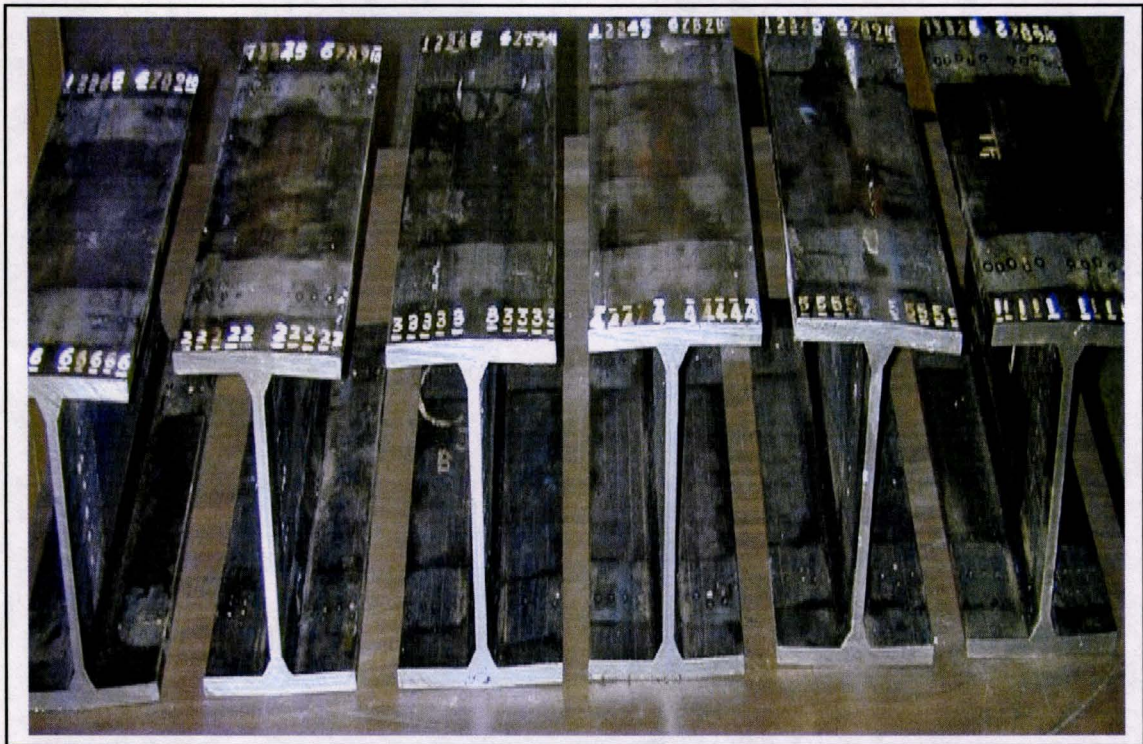
Figure 5.6: Specimens for Residual Stress Measurements
