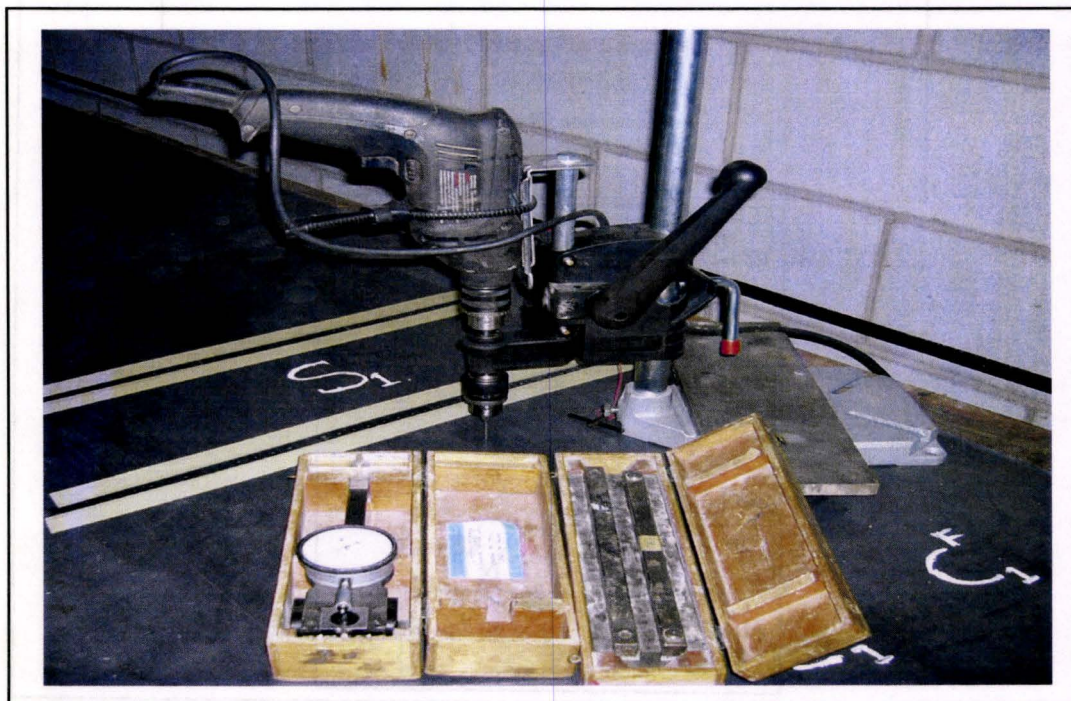
Figure 5.4: Gage Hole Drilling Assembly
