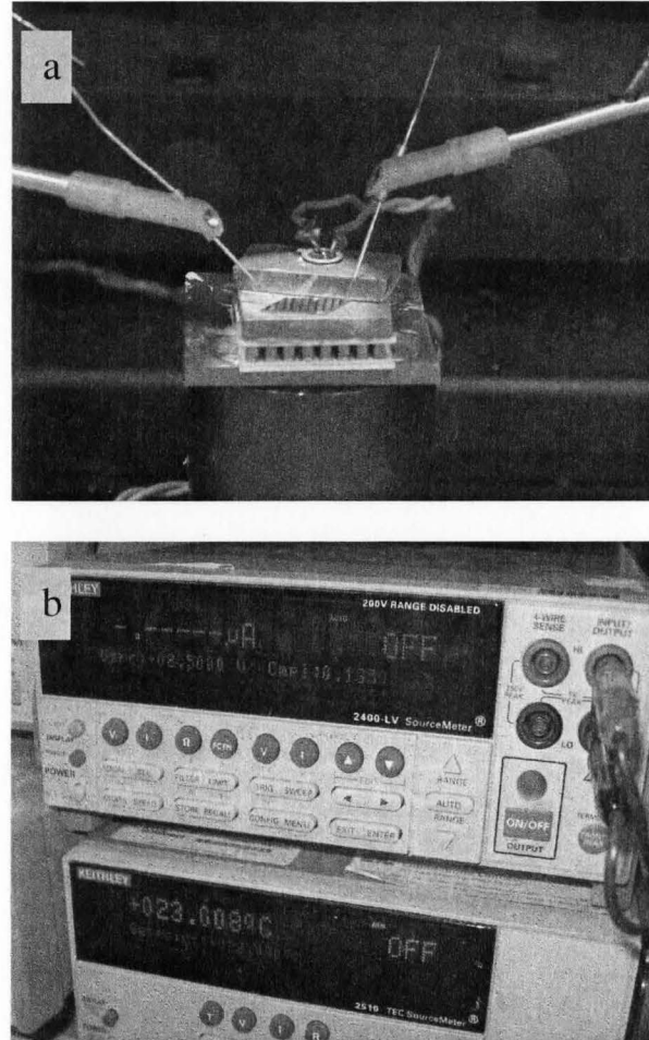
Figure 3.9. (a) The I-V measurement station showing the sample placed on a movable stage with the top and bottom contact probes and light illumination from top. (b) The Keithley 2400 LV source meter.
