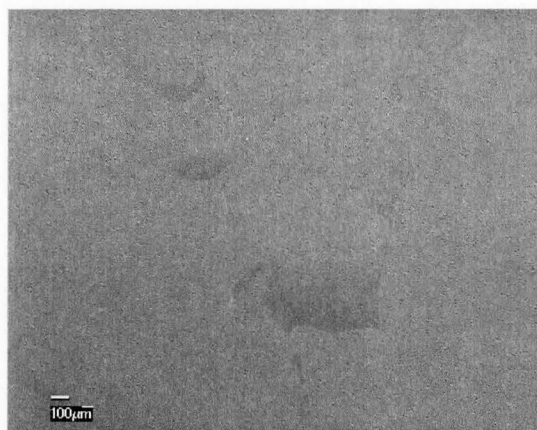
Figure 4.3. SEM image of S1818 spin-coated onto ITO-coated PET. The darker portions are the only places where S1818 has wetted the surface.
