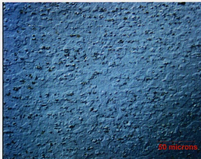
Figure 7.25: Microstructure of 75% deformed Al-Mg-Fe-Mn (15) alloy, annealed and quenched from 225 deg.C
