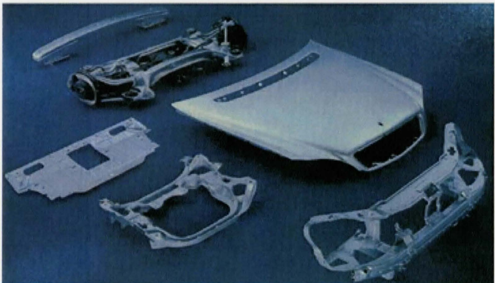
Figure 2.1: Aluminum parts of the S-class Mercedes (Daimler Chrysler) made of Al-Mg-Mn alloys ( www.key-to-metals.com )
