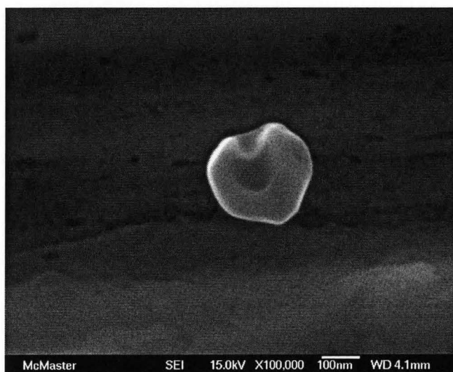
Figure 3-2: SEM image of YSZ particle before electrodeposition
