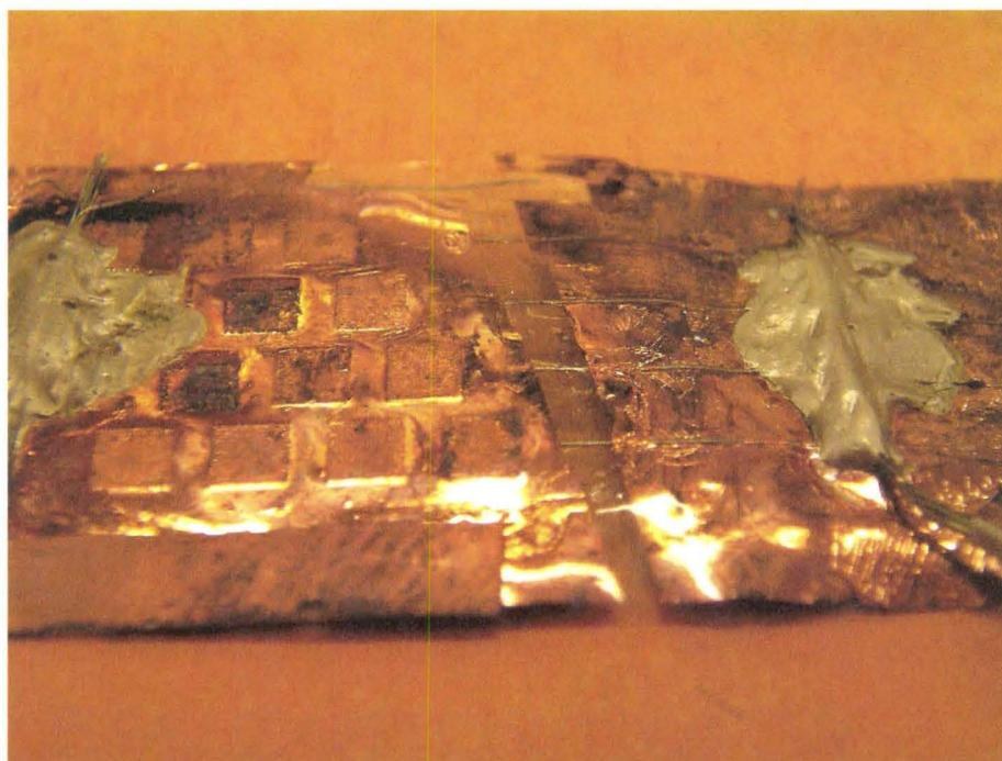
Figure 3.2: Backside view of flexible silicon solar cell sample in this thesis
