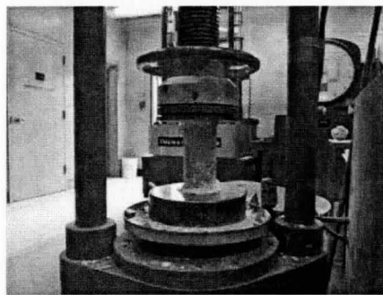
Figure 3.7: Tinius Olsen Universal testing machine 600-KN used to test the concrete 28-day compressive strength
