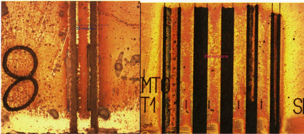
Figure 4-10: Optical images of damaged cantilevers after laser machining
