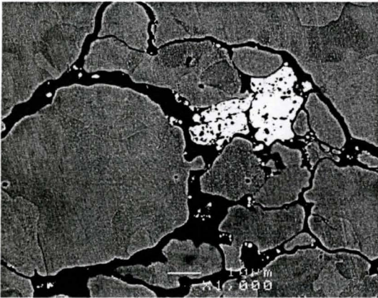
Fig. 3-40d. 1000X SEM - 2XF-Ni/2Cu/0.8C steel sintered @ (from left to right) 500°C, 800°C, and 1120°C.
