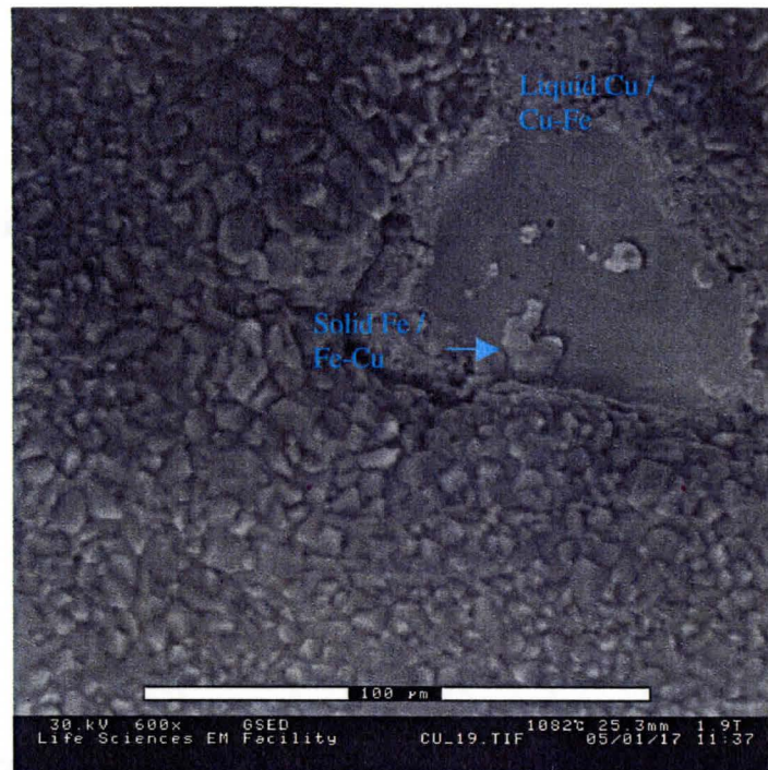
Figure 3-59. E-SEM image of sintering of 4Cu/0.5C steel at 1083°C.
