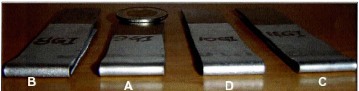
(b) >90^\circ bend test result edges are intact (c) >90^\circ inner side is intact
