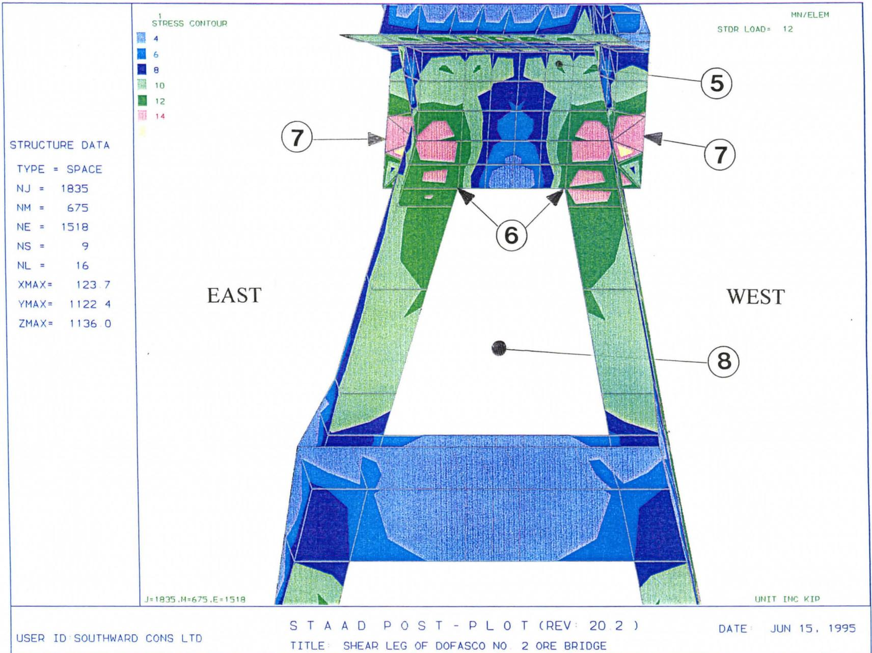
**FIGURE 68: Finite element analysis results at the base of the South Leg in its original configuration as viewed from above. (See text for notes)**
