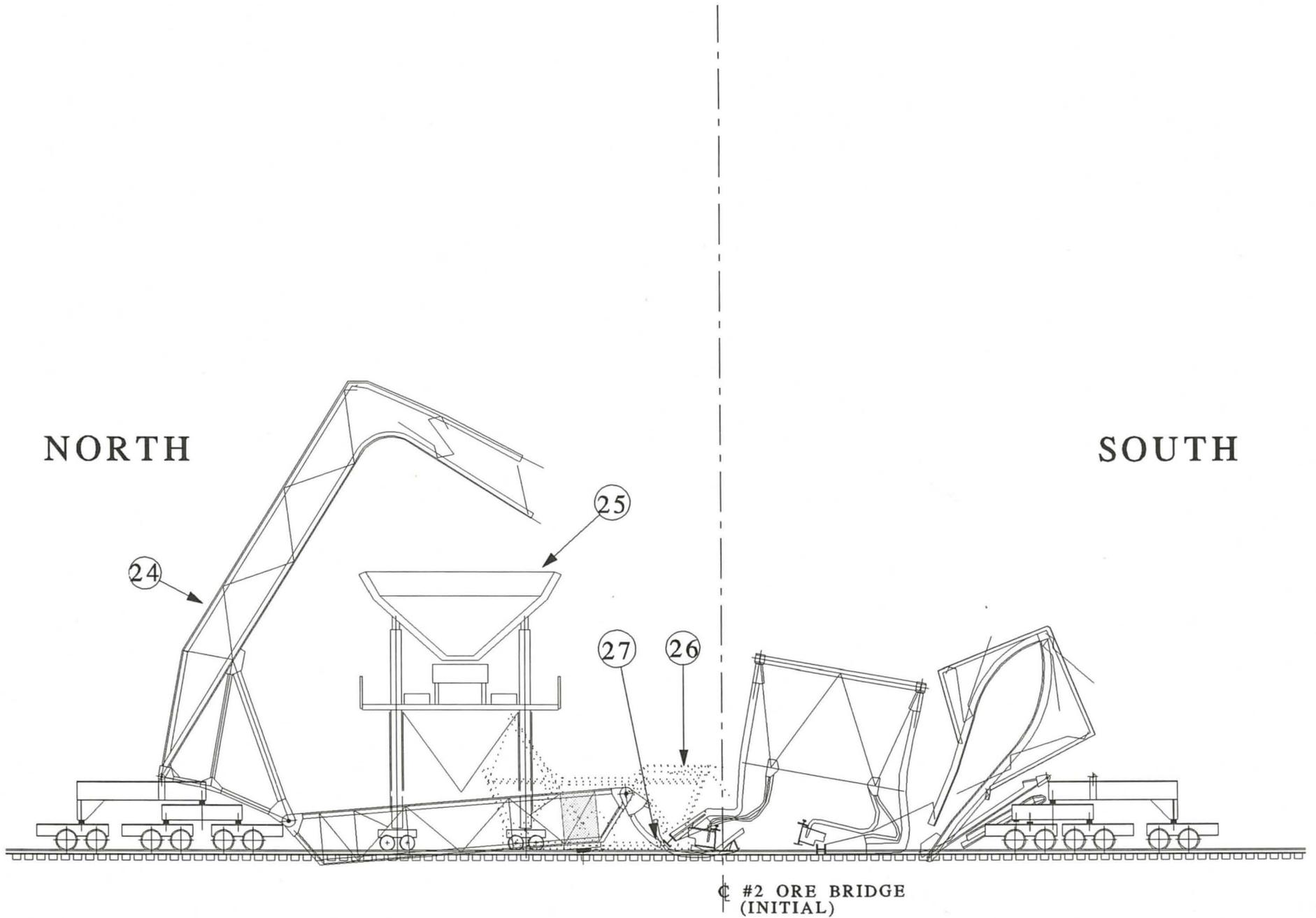
**FIGURE 43: Collapse of Shear Leg of No.2 Ore Bridge (looking east).
