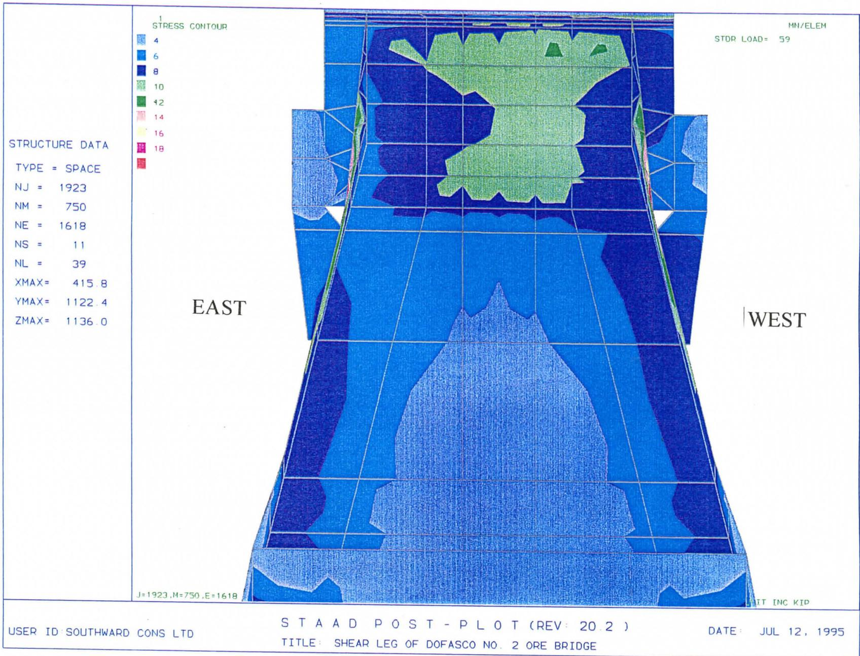
**FIGURE 77: Finite element analysis results at the base of the South Leg including the effect of the unbalanced honner loading**
