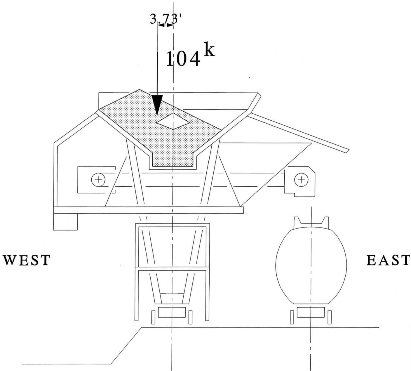
**FIGURE 63: Hopper live load when it is filled off-centre.**
