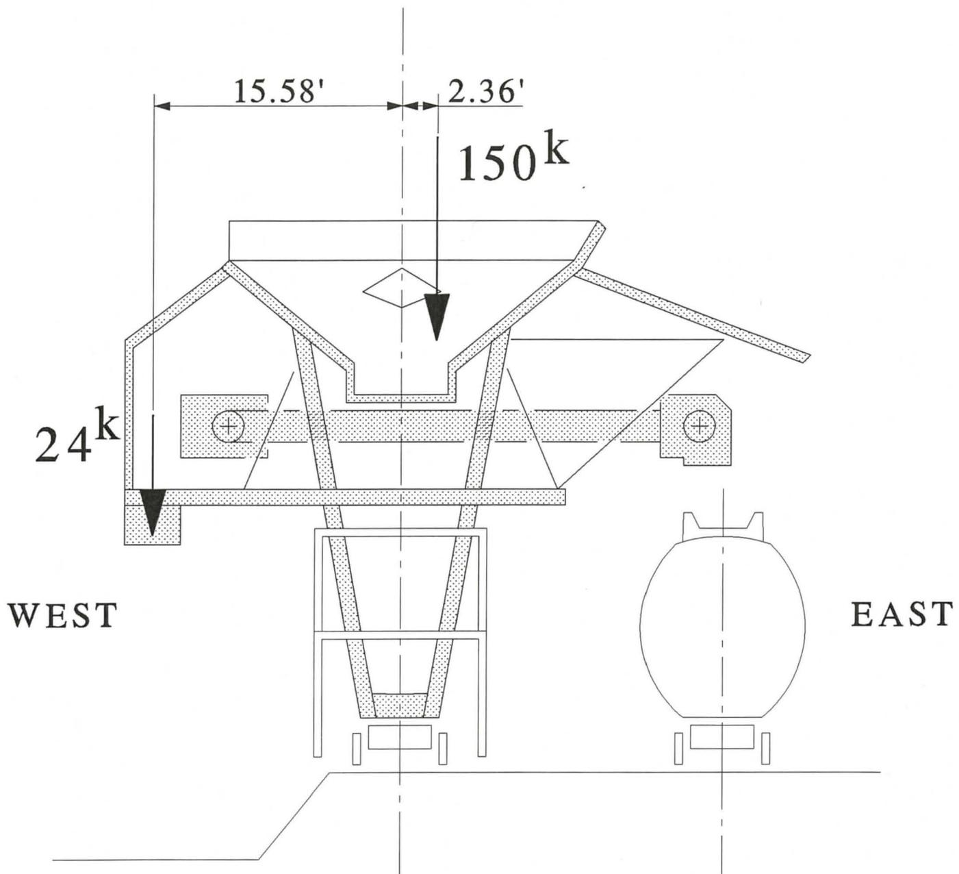
FIGURE 58: Hopper dead loads including the counterweight.
