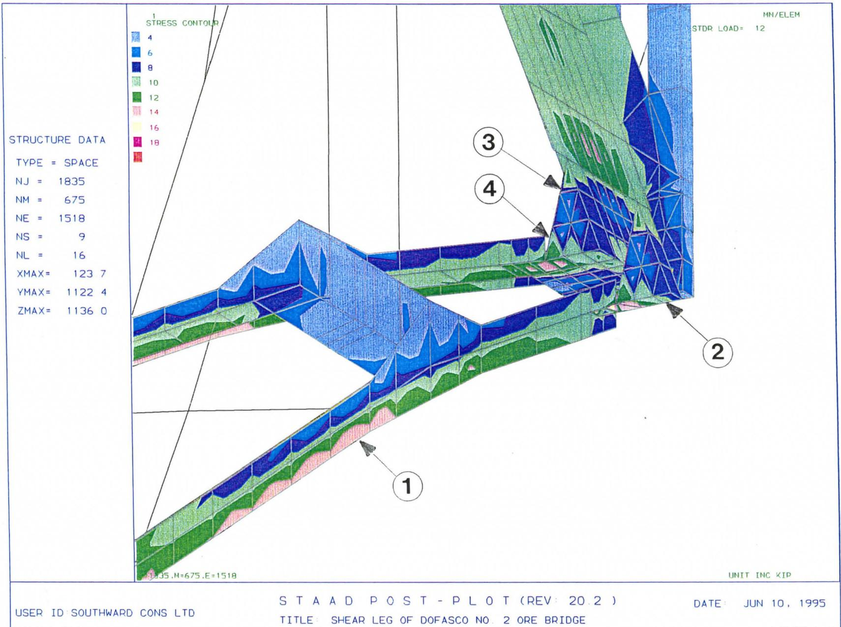
**FIGURE 67: Finite element analysis results at the base of the South Leg in its original configuration. (See text for notes)**
