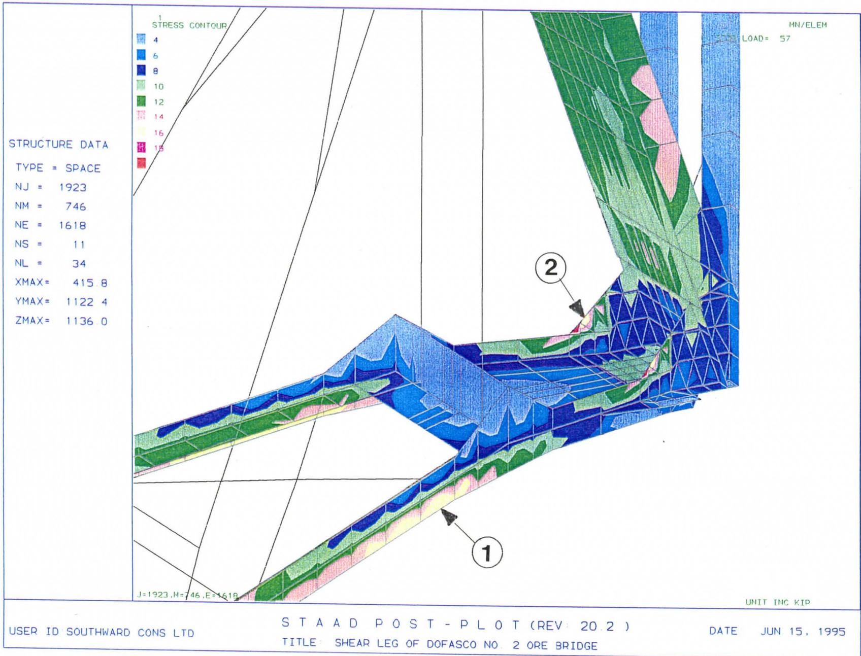
**FIGURE 73:** Finite element analysis results at the base of the South Leg of the Shear Leg once the additional reinforcements were added. (See text for notes)
