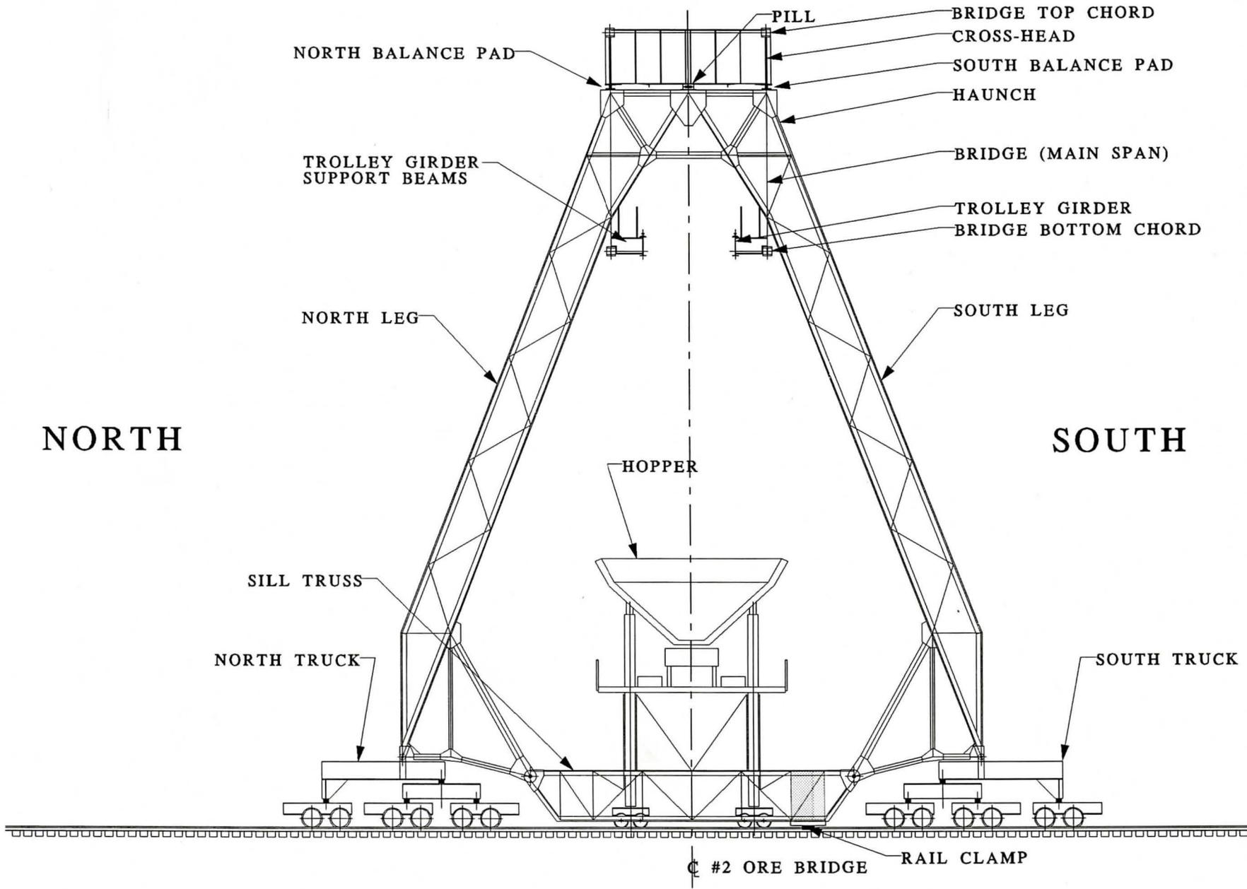
FIGURE 15: No.2 Ore Bridge Shear Leg (looking east).
