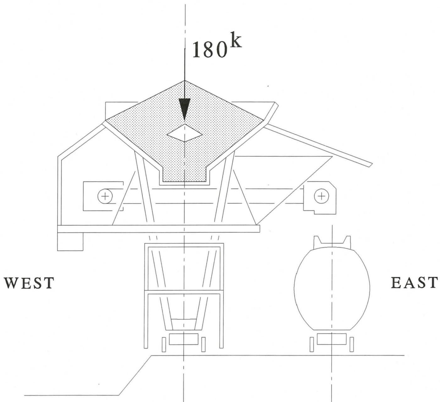
**FIGURE 61: Hopper live load when completely filled.**
