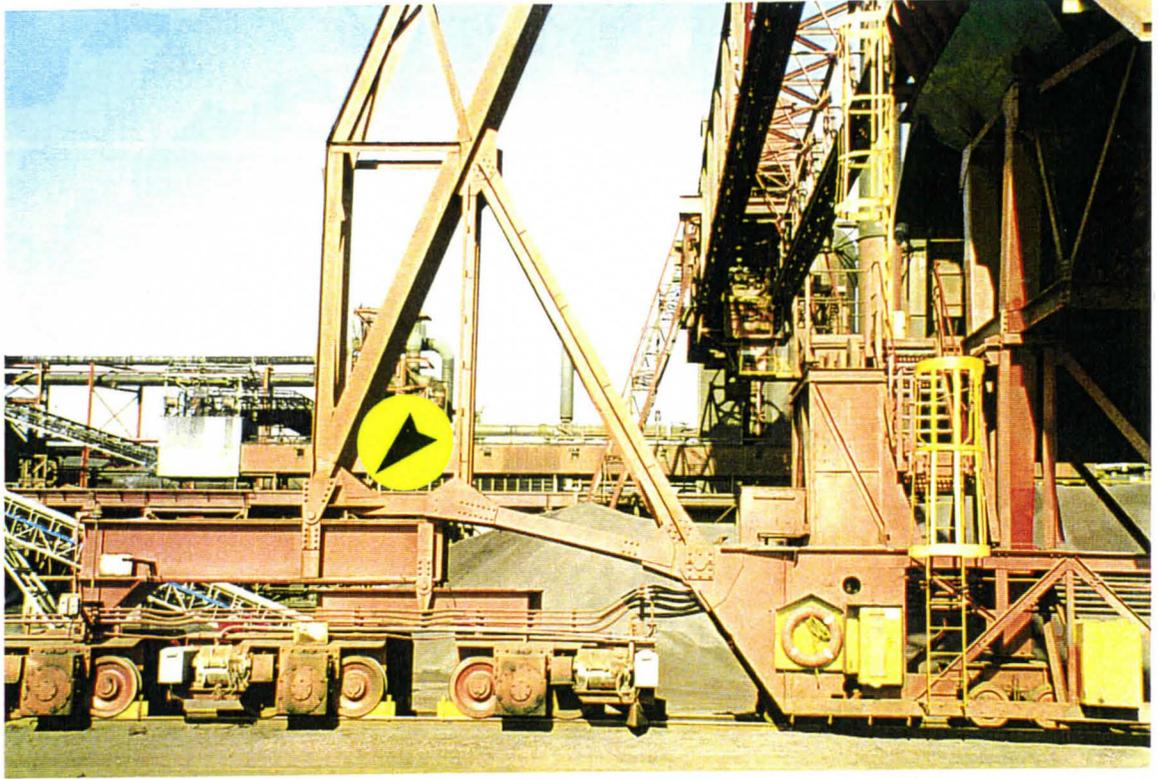
**FIGURE 71:** View of base of South Leg of Shear Leg of the No.1 Ore Bridge. (Arrow notes the gusset extensions which were added)
