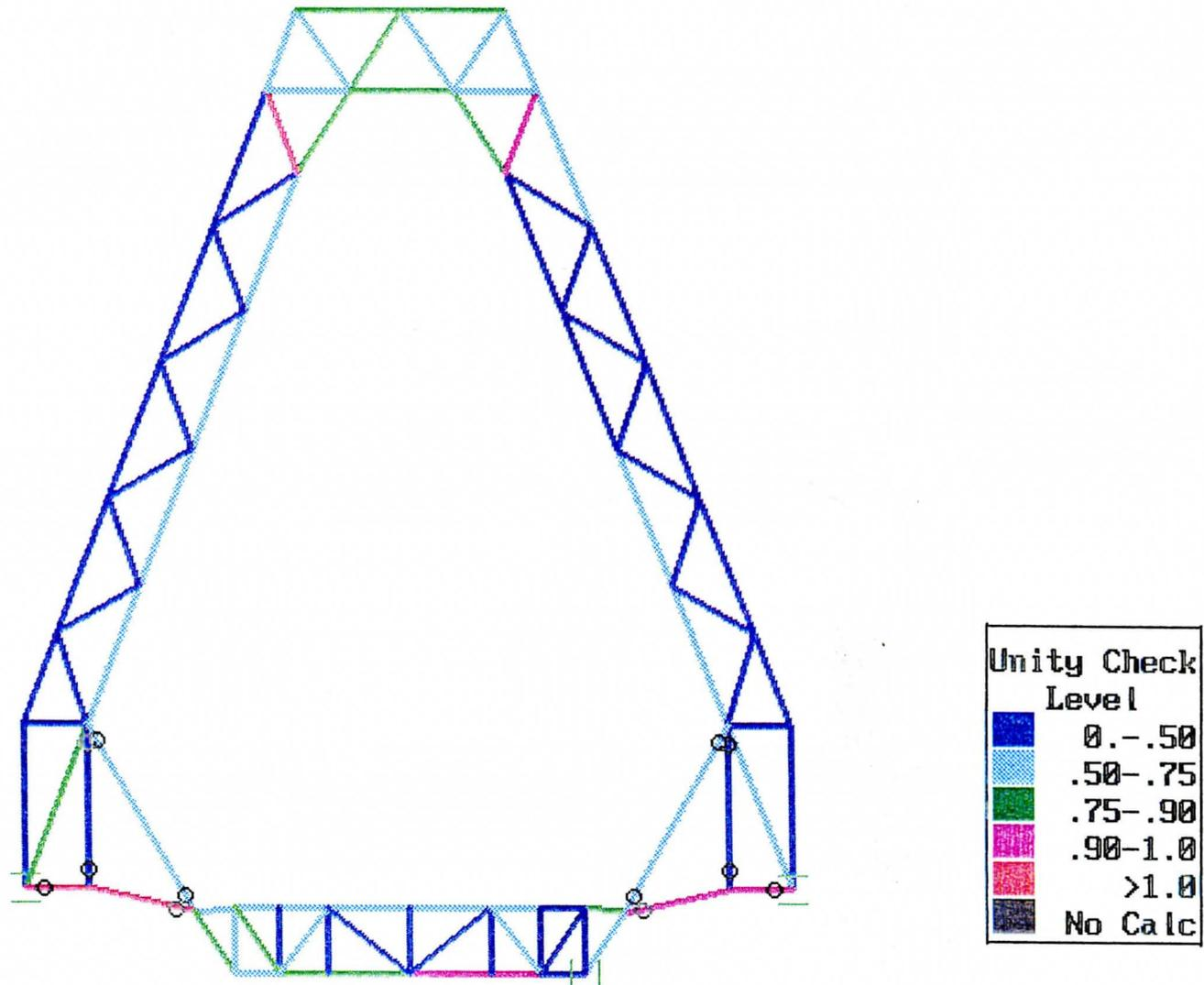
**FIGURE 65:** Results of a two-dimensional structural design check of the Shear Leg of the No.2 Ore Bridge with the hopper addition.
