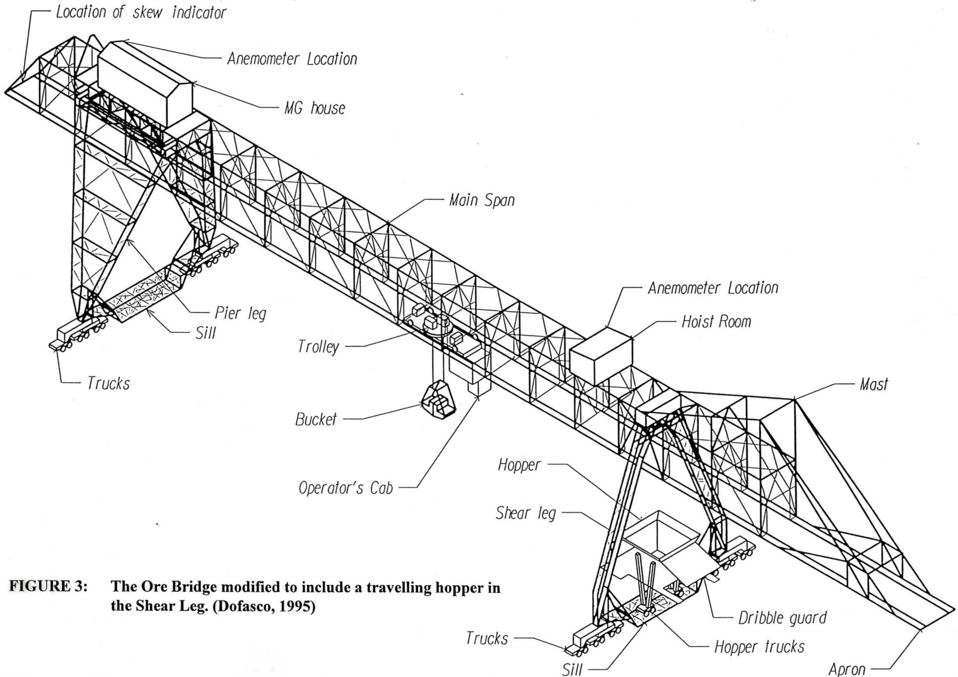
**FIGURE 3: The Ore Bridge modified to include a travelling hopper in the Shear Leg. (Dofasco, 1995)**
