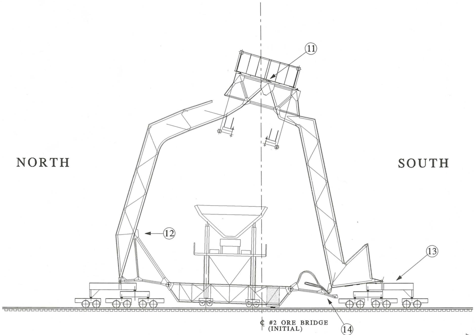
**FIGURE 35: Collapse of Shear Leg of No.2 Ore Bridge (looking east).
