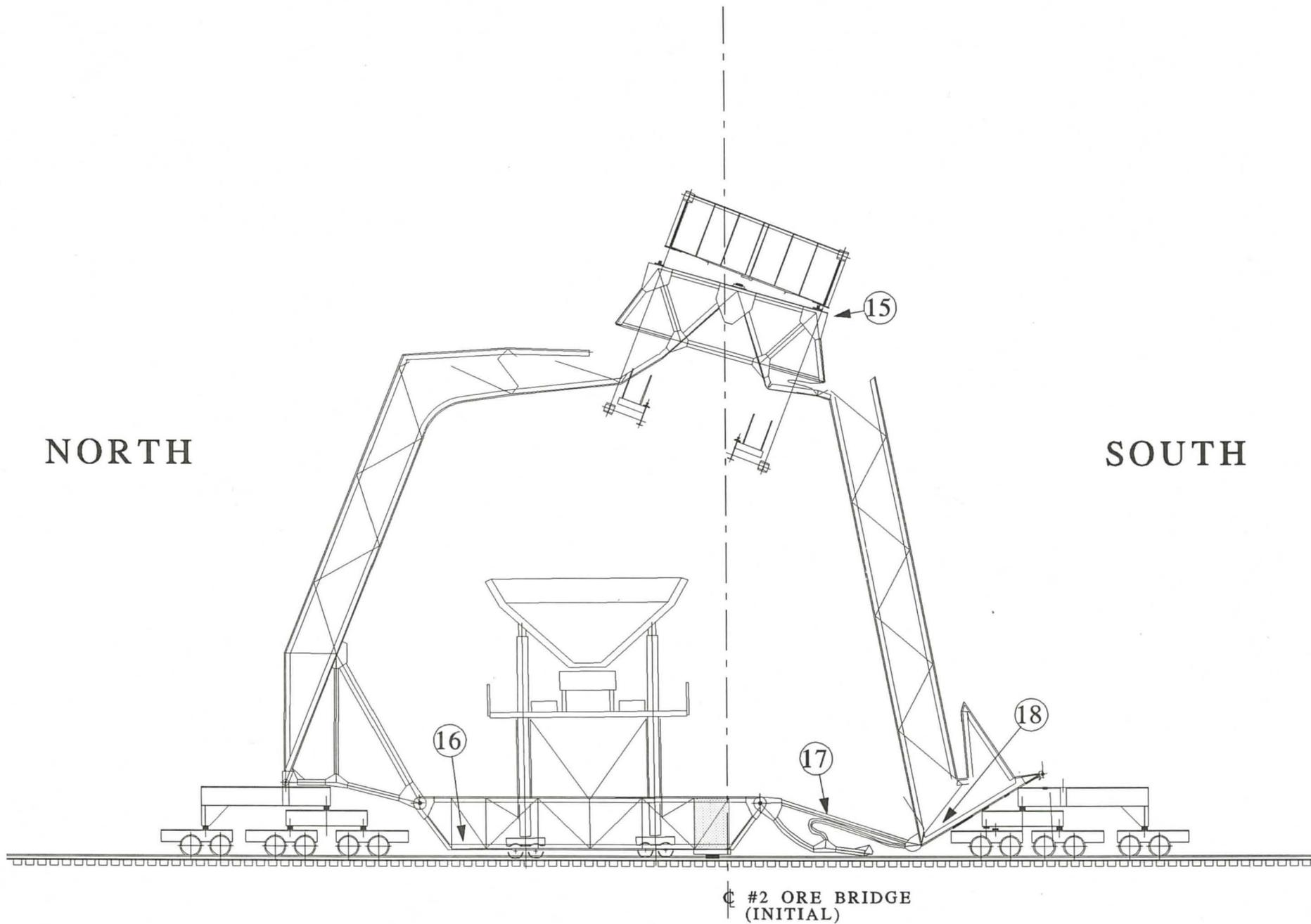
**FIGURE 36: Collapse of Shear Leg of No.2 Ore Bridge (looking east).
