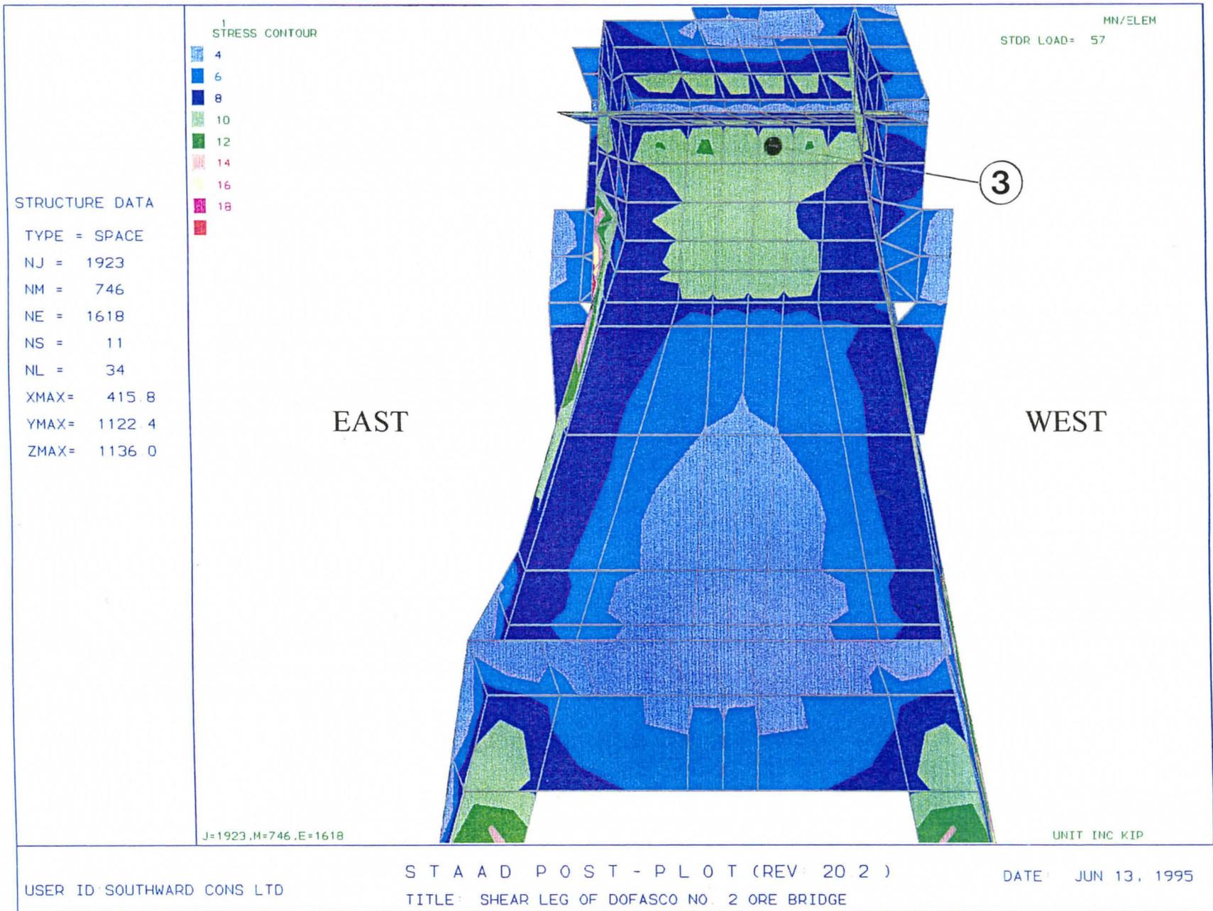
**FIGURE 76:** Finite element analysis results at the base of the South Leg including the additional reinforcements under gravity loading. (See text for note)
