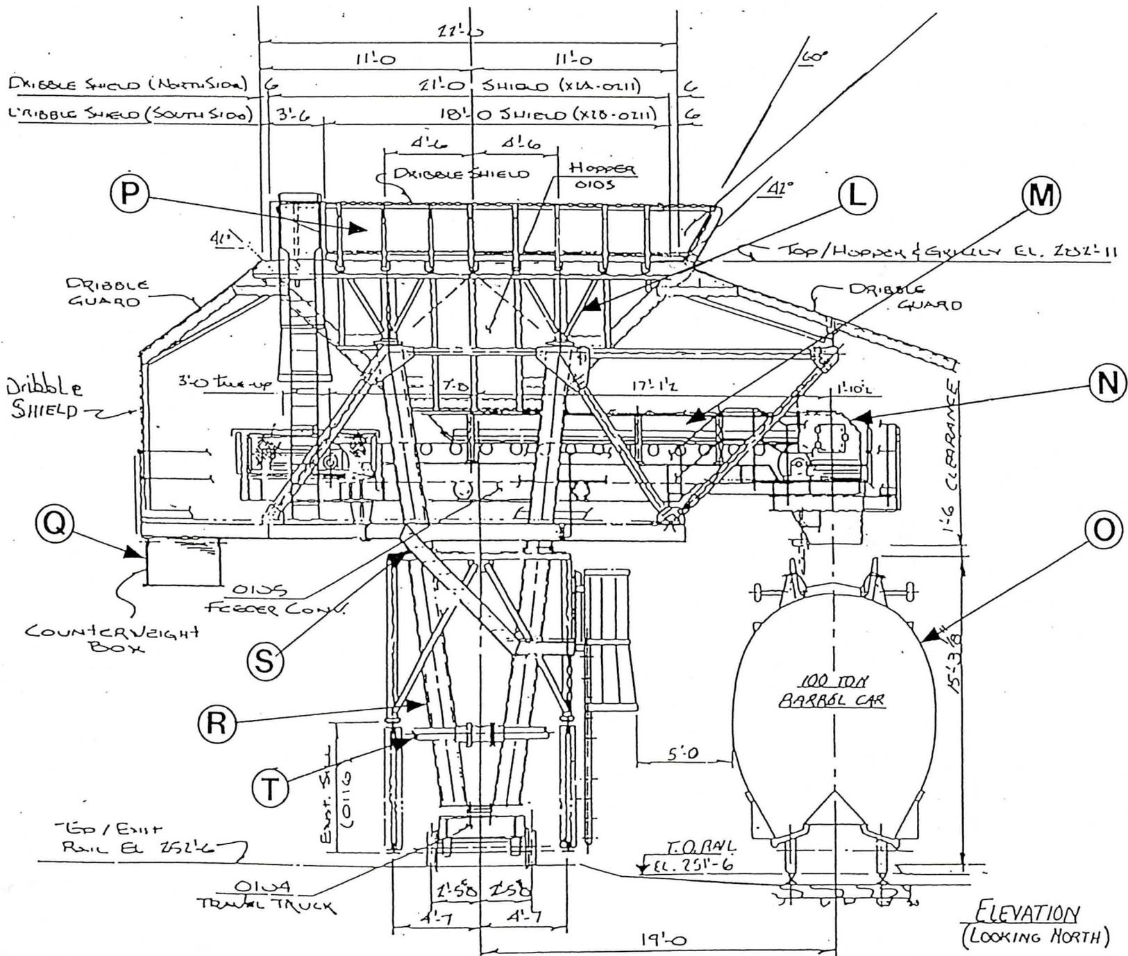
**FIGURE 4: General Arrangement of the hopper (looking north).**
