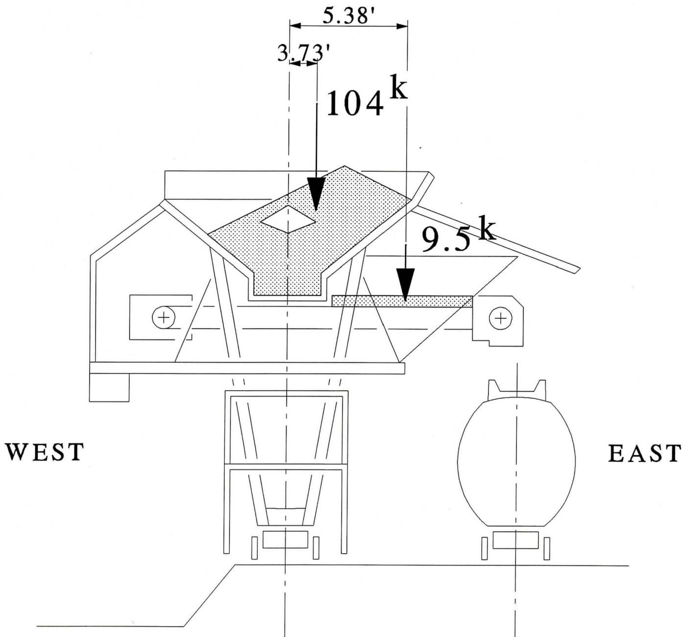
**FIGURE 64: Hopper live load when it is being emptied.**
