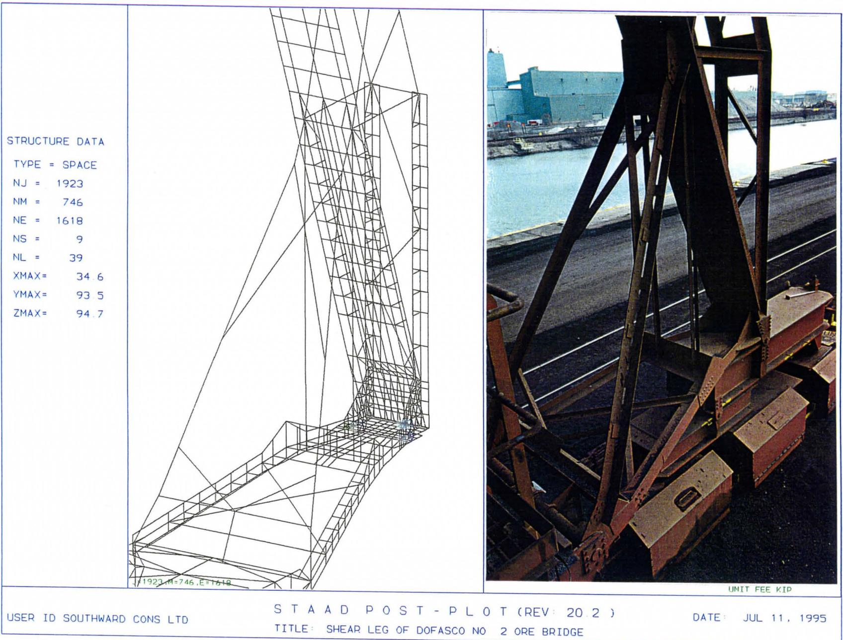
**FIGURE 66b:** Closeup of finite element mesh at the base of the South Leg of the Shear Leg.
