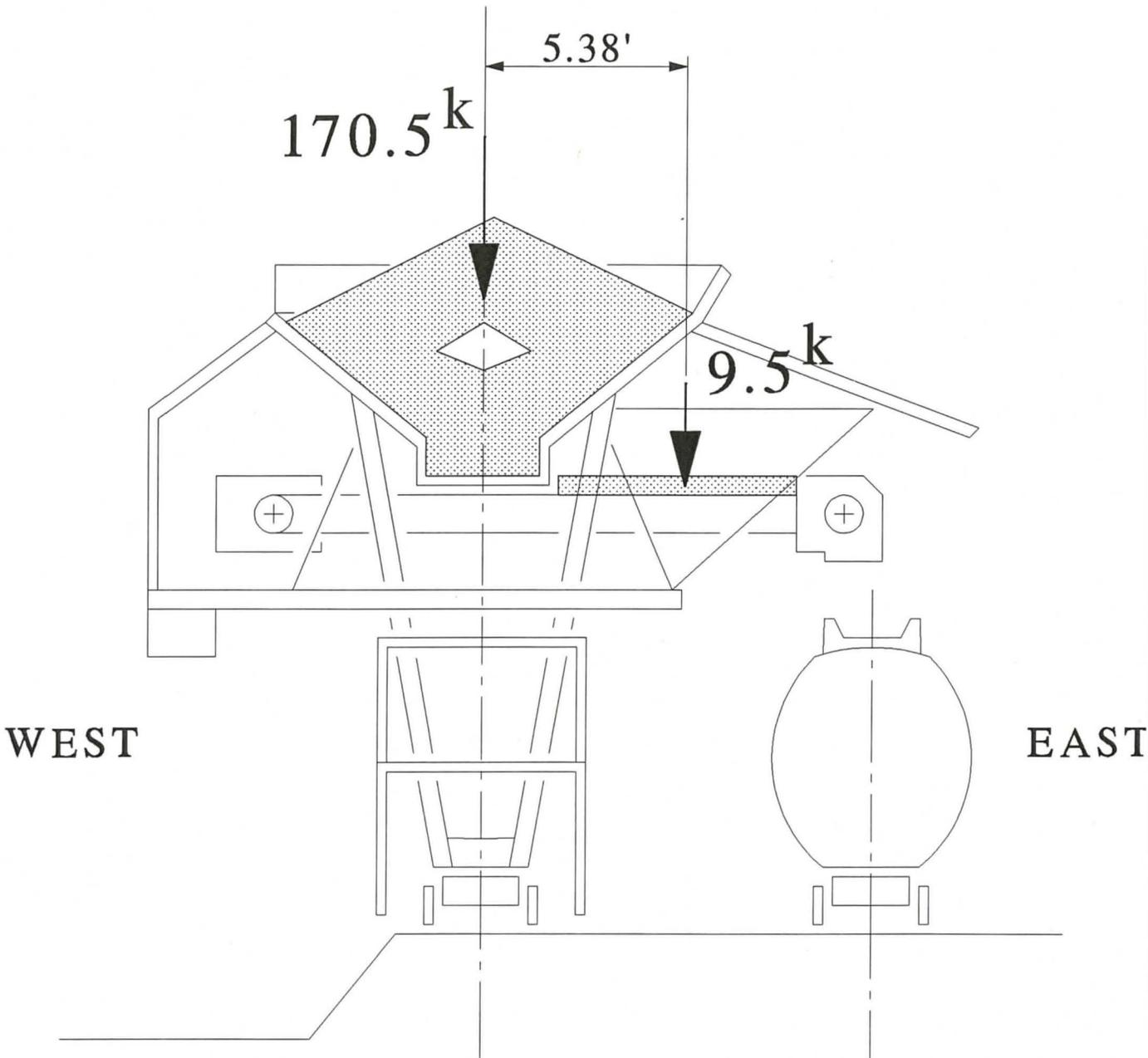
**FIGURE 62:** Hopper live load when hopper is just beginning to be emptied.
