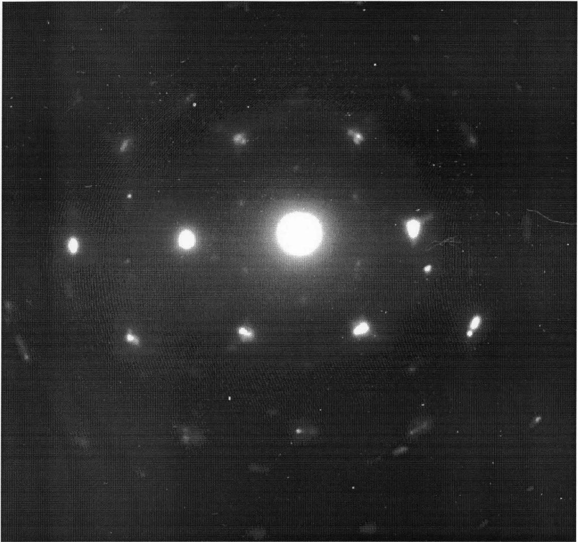
**Figure 4-21 TEM Ring Pattern Associated with an Amorphous Film**
