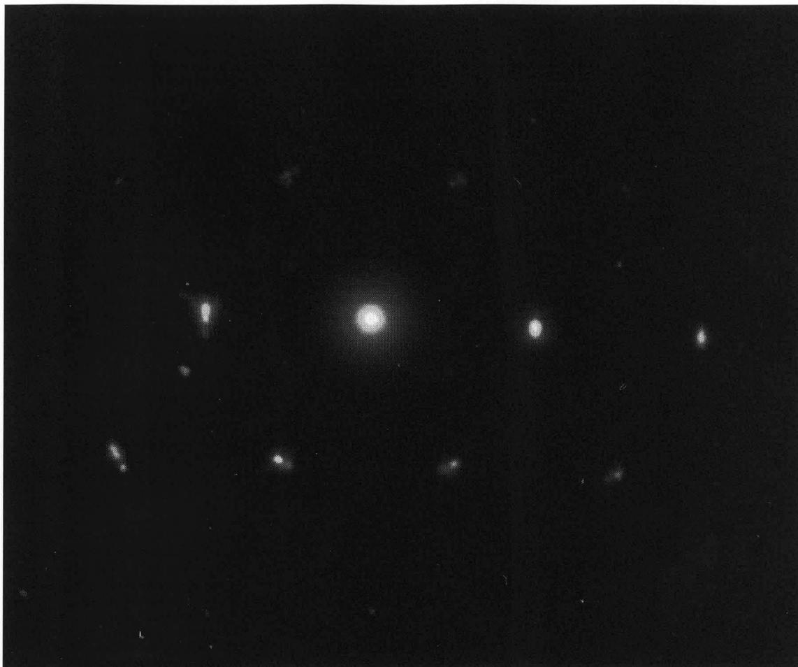
**Figure 4-20 TEM Diffraction Pattern of Nickel Induced Crystallized Silicon Film**
