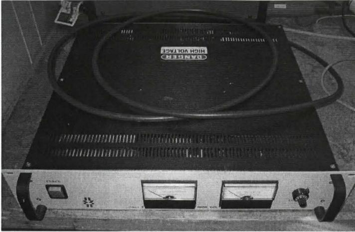
Figure 4.8: Glassman high voltage for dc applications
