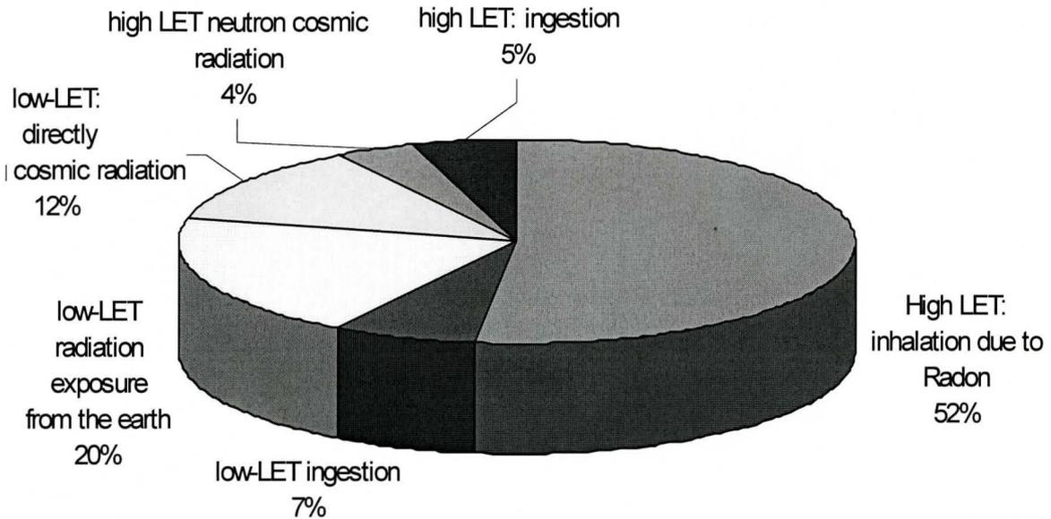
Figure 2. Sources of natural radiation on the earth. LET is linear energy transfer. (BEIR, 2006)
