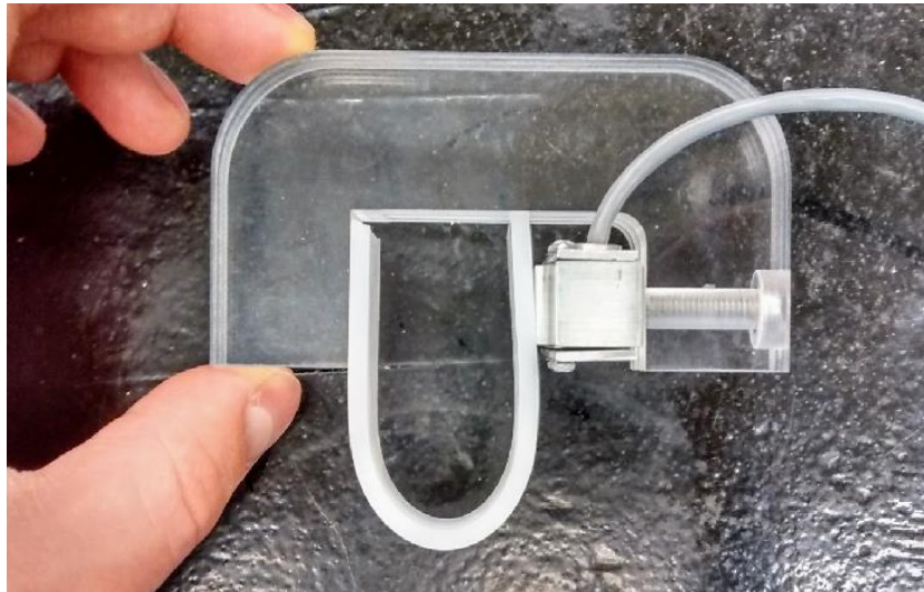
Figure 31: Acrylic sample retaining device with fitted OMEGA sensor to read forces in a compressive manner.
