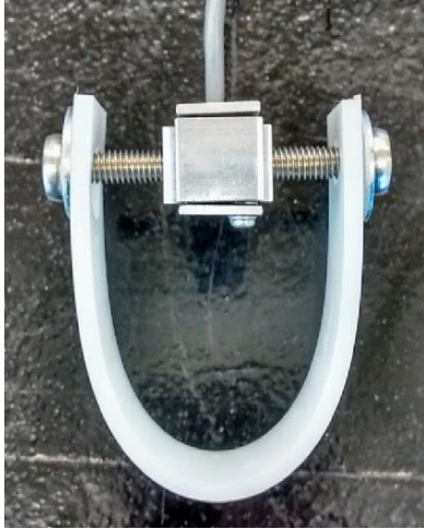
Figure 26: OMEGA sensor with mounted polymer sample.
