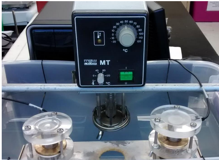
Figure 15: ESCR Test used to identify possible sample derived acoustic activity.
