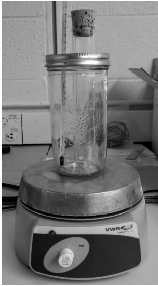
Figure 11: Simplified Mason jar testing configuration.
