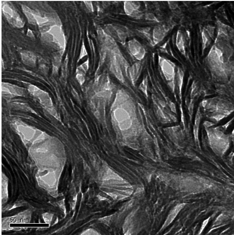
Figure 6.6: Ion milled bovine femur cut parallel to the long axis. The open structure is preserved by ion milling.
