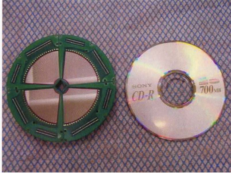
Figure 4.10: The CD detector in our lab & a real CD disk.
