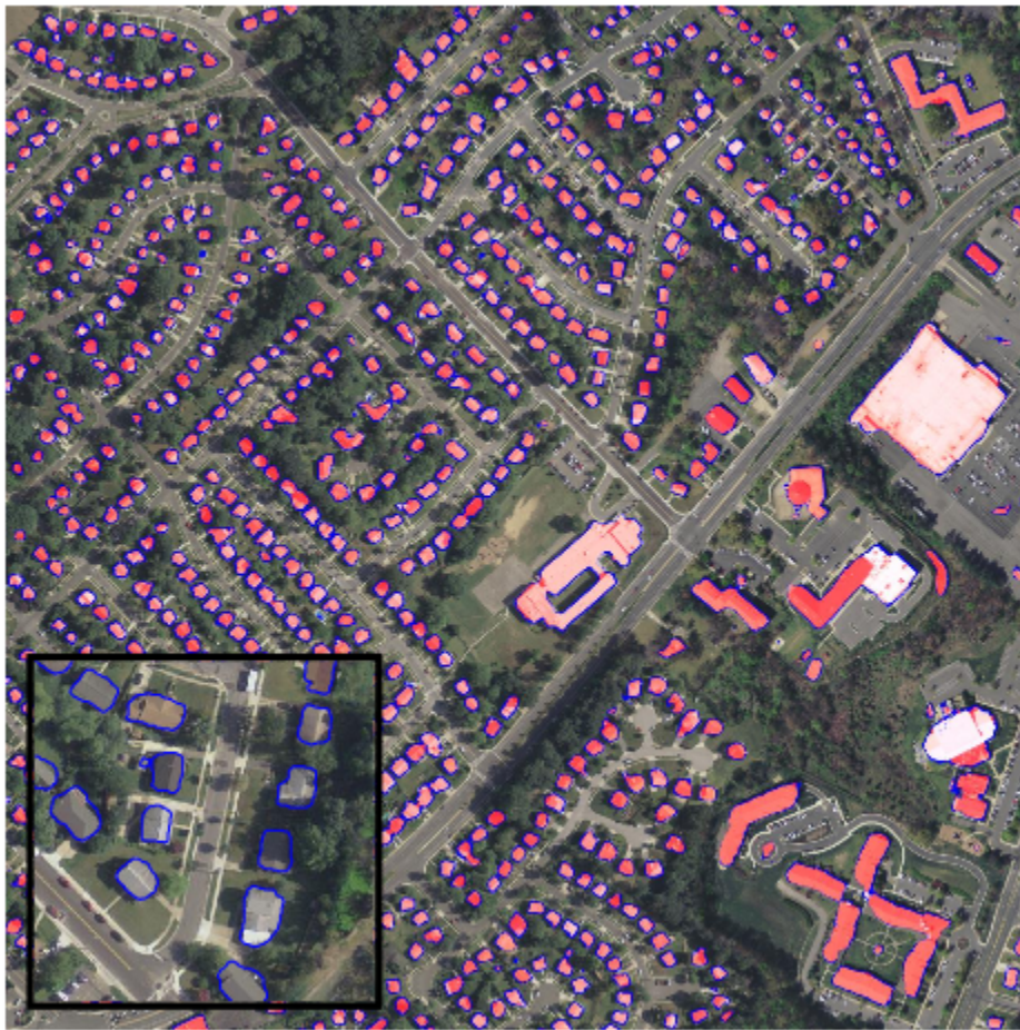
Figure 6.2: Example of the convolution network developed by Yuan (2016) in a residential area from Washington, D.C.. Transparent red areas represent the infrastructures extracted using the convolution network and the blue pixels indicate the boundaries (Yuan, 2016).
