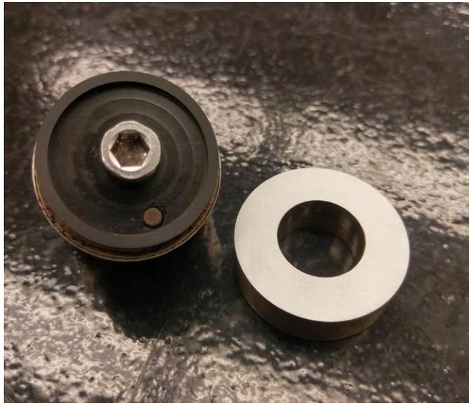
*Figure A3 - Unworn polymer sample and C1018 Washer*
