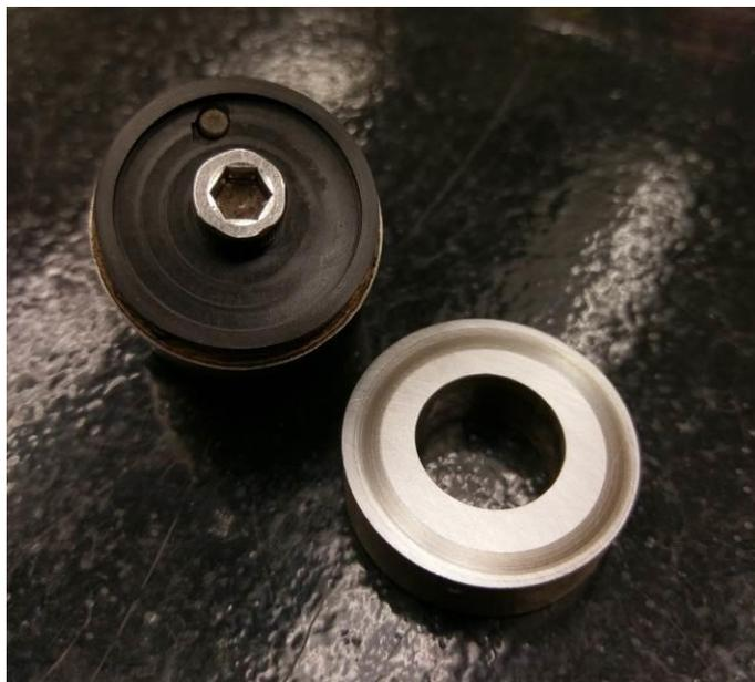
Figure A4 - Worn polymer sample and C1018 washer.
