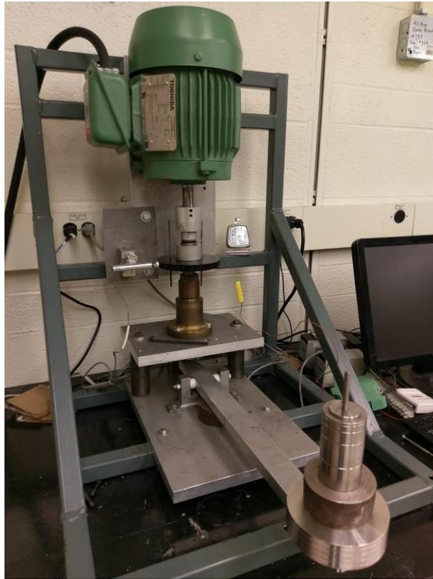
*Figure A1 - Tribometer fabricated specifically for this study.*
