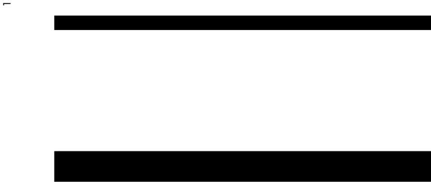
**Figure A-3.** Digital mask for the inkjet printing pattern of SU-8 films (2 cm in figure = 1 cm in real device).
