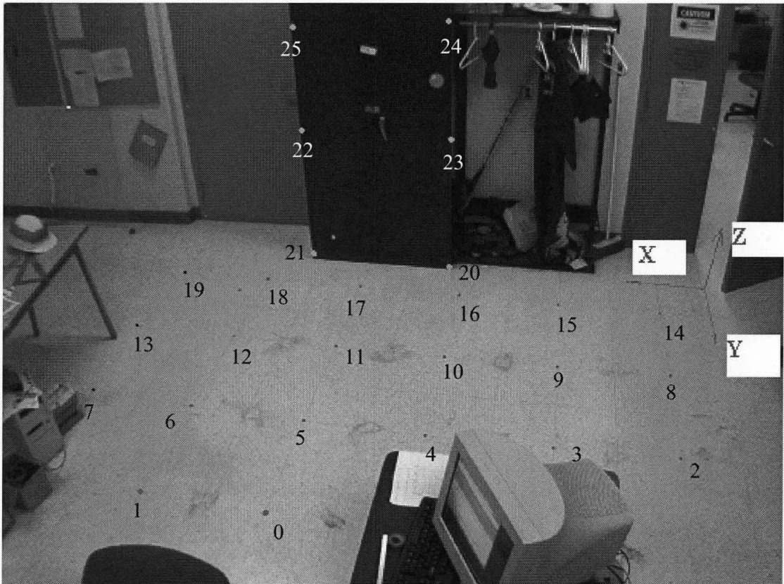
Fig. D.5. Camera Calibration picture with 26 calibration points.
