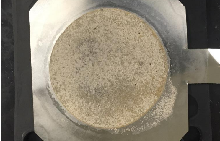
Figure S 5 SSF cathode image after 5-day fed-batch SSF MEC operation for Set D
