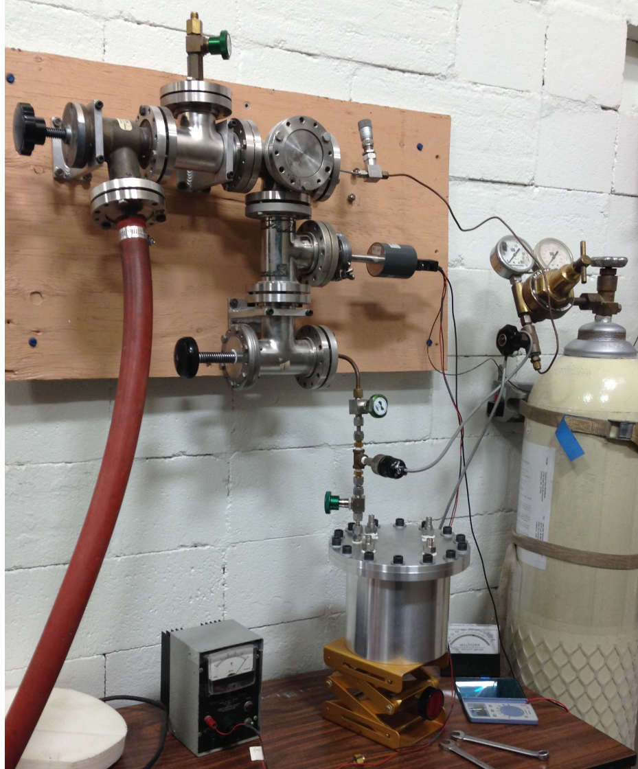
Figure 4.8: The vacuum set up used with the prototype THGEM-based TEPC. The vacuum was made with a rotary vane vacuum pump. After vacuuming, the detector was filled with propane-based tissue equivalent gas at the pressure of 49.1 torr to simulate the energy loss pattern of charged particles in 2\ \mu\text{m} of soft tissue.
